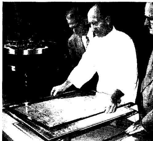
Figure 6.—The bronze bracket around the edge of the cover glass holds the assembly of backing paper, document, and cover glass in position in the enclosure. The bracket also serves to keep the document away from the area heated by soldering during the final sealing operation. Left to right: Mr. A. W. Kremer, Dr. R. W. Wampler, and Dr. G. M. Kline.
