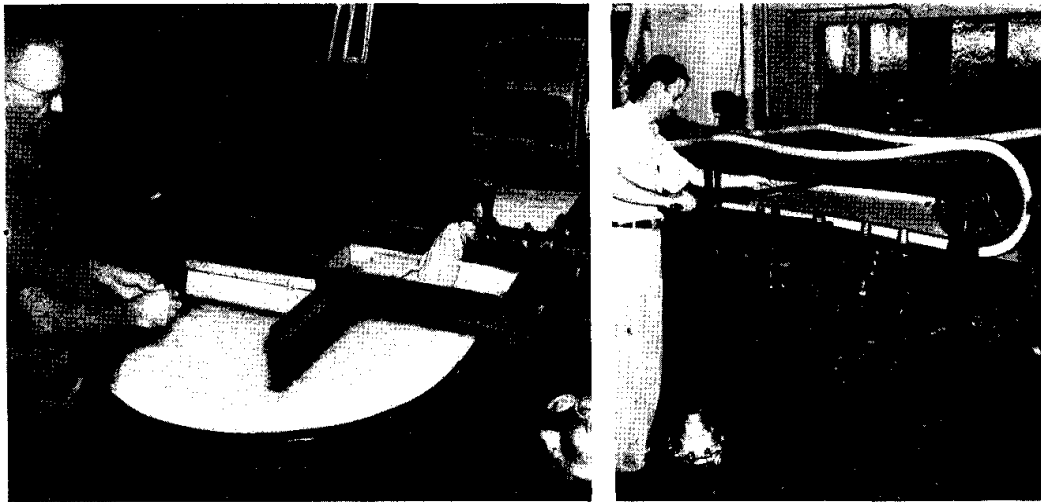
Figure 20.—The beater in the experimental paper mill at the National Bureau of Standards, in which the paper stock for the backing paper was prepared from cotton rags. The special backing paper serves as a physical protection and moisture reservoir without contaminating the documents (left). The experimental paper-making machine at the Bureau, on which the backing paper was made for use in the preservation of the Declaration of Independence and the Constitution of the United States in glass enclosures filled with helium (right).
