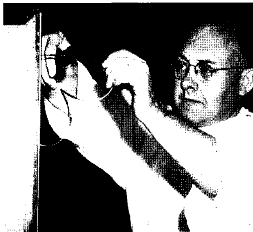
Figure 15.—The air in the document enclosure is flushed out with humidified helium for several days until a reading taken with the leak detector indicates that the air has been completely driven from the capsule and the unit is ready to be sealed. Then the copper inlet and outlet tubes are constricted and cut with pliers.
