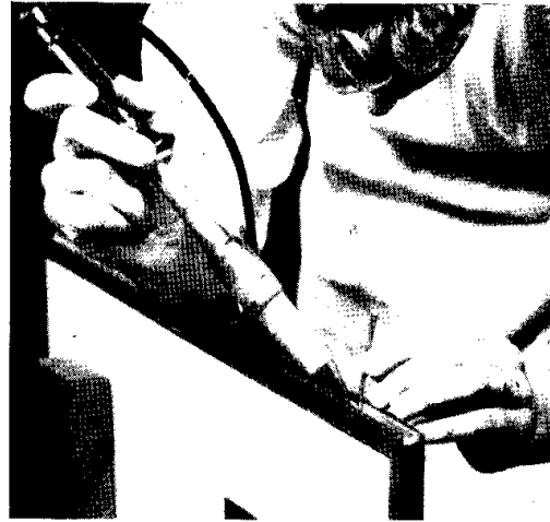
Figure 16.—The constricted tubes, which extend through the lead strip, are removed from the strip and the holes sealed with solder. The facsimile document is now entirely sealed within the test enclosure.
