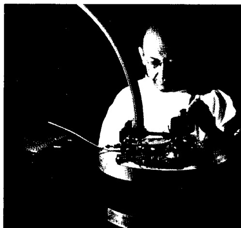
Figure 13.—The pure helium is humidified by adding sufficient water vapor to produce a relative humidity of 25 to 35 percent. The proper humidity is achieved by passing the helium through distilled water maintained at a temperature of 4° to 6° C. The insulated water bath, in which the humidification tower is immersed, is thermostatically controlled at the desired temperature. Dr. G. M. Kline and Mr. E. C. Creitz are checking the temperature of the bath.
