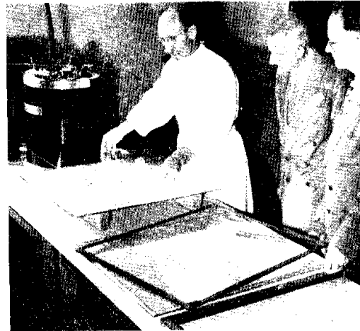
Figure 4.— With the document in position, the cover glass is placed over it to keep it from wrinkling. On the table, ready for succeeding steps in the test sealing are the bronze bracket and front glass plate (center), and the bronze outer frame (extreme right).
