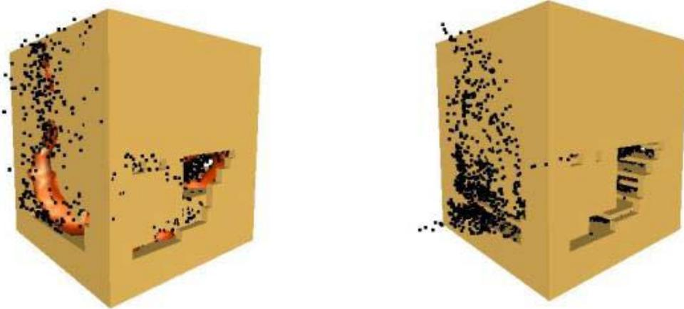
Figure 5: A comparison of two simulations of the fire in the north tower, with very different assumed internal damage geometries and fuel distributions. The left simulation shows very large flames extending from the damage holes, whereas that at the right shows little flame extending out of the exterior damage holes. The simulation on the right seems to agree much more with pictorial records, indicating that these postulates are better.
