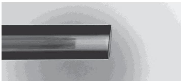
Angle-cleaved fiber showing typical size of remaining collapsed region (optical microscope image).
