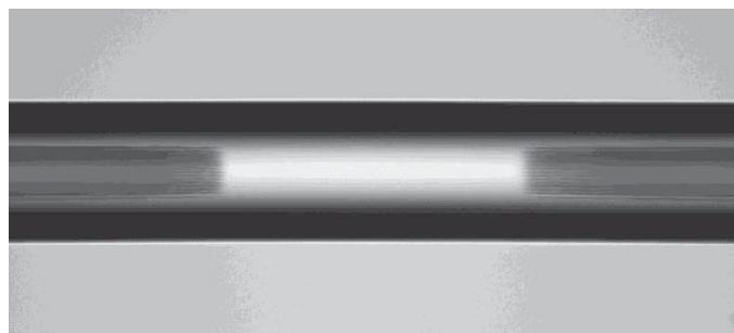
Collapsed region (bright in center) of fiber, with photonic crystal holes visible to left and right of collapsed region (optical microscope image).
