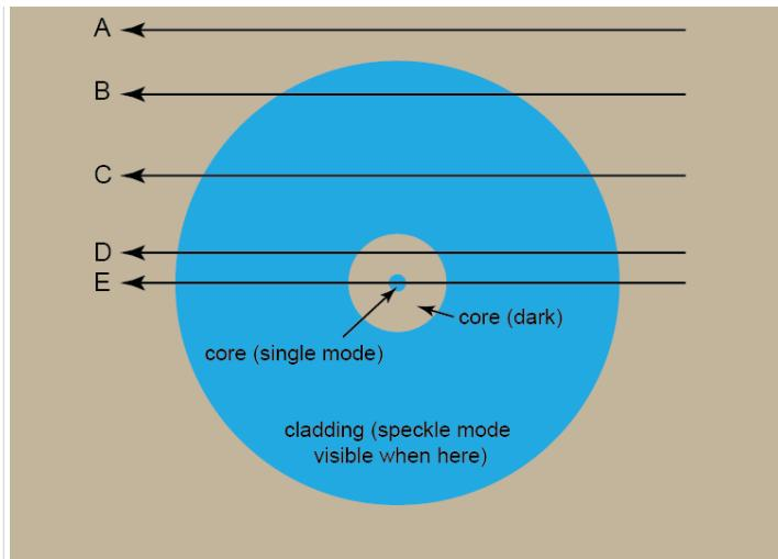
Finding the single mode. Image shows the fiber facet, five different sweep positions for an input beam, and regions of the facet where different modes are excited. If the facet is not at the focus of the lens, the input beam will have a large area and may excite both the single mode and the speckle mode at the same time, making it more difficult to see the single mode.
