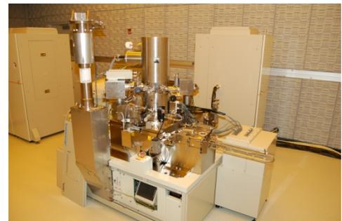
The new [Heidelberg DWL 66FS maskless laser lithography system](#) is also about to become fully available in the cleanroom. Tool managers [Rich Kasica](#) and [Marc Cangemi](#) are working toward placing the Heidelberg on Coral-ready status in early May. The Heidelberg will also get a new 4 mm, large-format write head soon which should reduce some image writing times by more than 50%.
