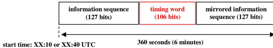
Figure 7 – Structure of 6-minute extended symbol
