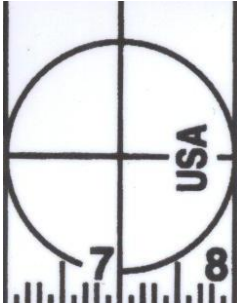
Figure 14: Circle-fitting was not performed on vendor C rulers since part of the circumference was obstructed by other printed features.
