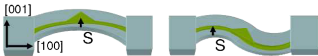
FIG. 1 (color online). Schematic of a bend applied to a QD in a nanobridge: (left) symmetric (biaxial deformation) bend with a QD at an antinode, and (right) vertical shearing bend with a QD at a node. S is the bend amplitude for clamped ends.
