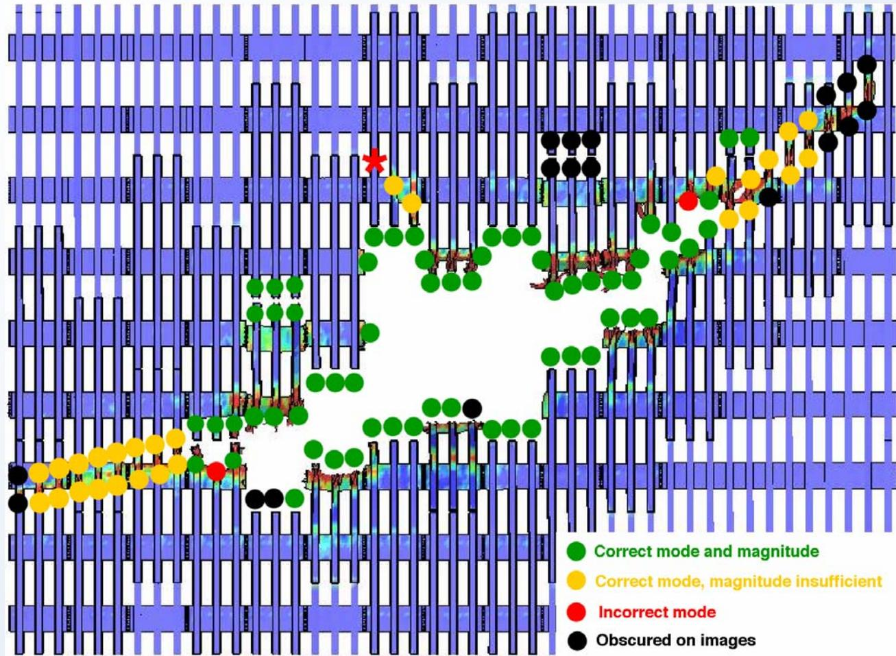
Comparison of observed and calculated base case impact damage to the north wall of WTC 1
