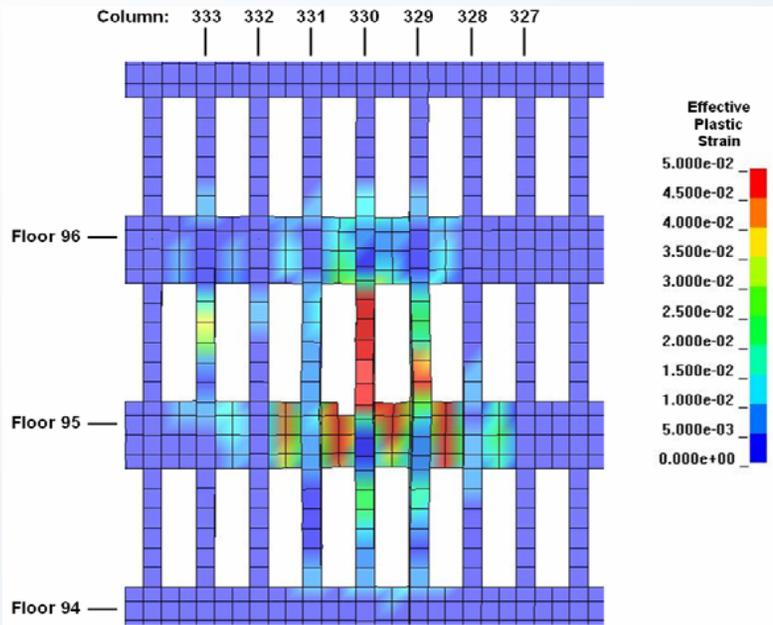
Calculated damage to the south wall of WTC 1
