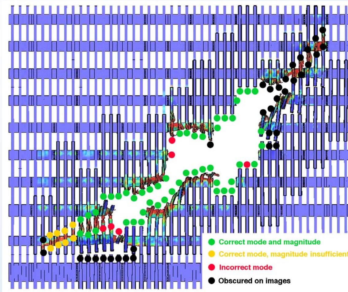
Comparison of observed and calculated base case impact damage to the south wall of WTC 2
