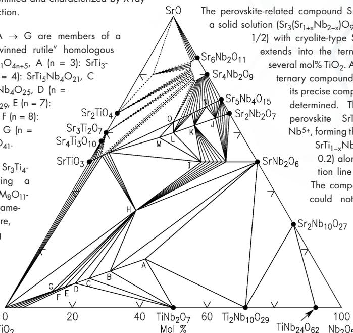
TiO<sub>2</sub>-Nb<sub>2</sub>O<sub>5</sub> system (Figs. EC-444, 9529). Phase I is a tetragonal tungsten bronze system, Sr<sub>6-x</sub>Ti<sub>2-2x</sub>Nb<sub>8+2x</sub>O<sub>30</sub>, with the value of x ranging from 0 to 0.5.
