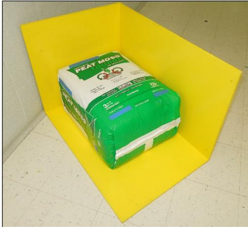
**Figure 3-1. Dimensional Measuring Frame**
