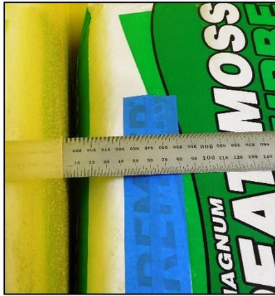
**Figure 3-3. The rigid frame allows the observer to hold the zero reference point firmly in place.**
