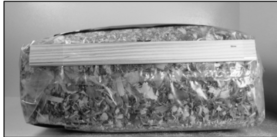
Exhibit 29. Plumped bedding package illustrating rounded edges (angles), which hinders getting accurate measurement points.
