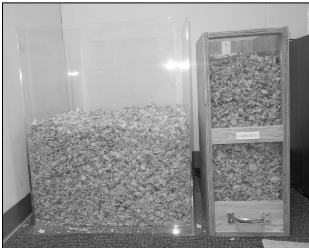
Exhibit 16. Test Measures Used in Study. The large test measures hold up to 279 L (10 cu ft) while the small measures hold up to 52 L (1.5 cu ft).
