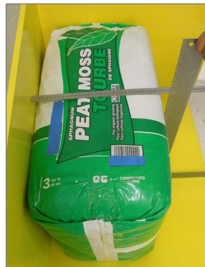
Exhibit 5. Width Measurement – the frame is rotated on its end to vertical so that the carpenter square does not compress the product.
