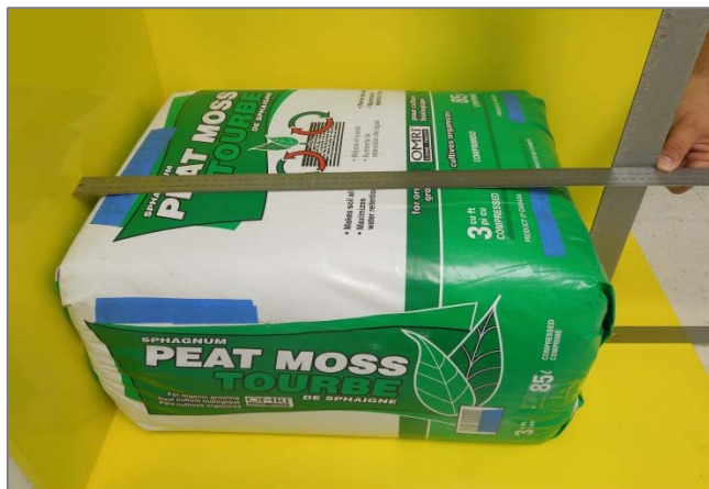
Exhibit 4. Height Measurement – A packaging tail on the end of the package can affect this measurement so it has been folded over and taped against the end of the package.
