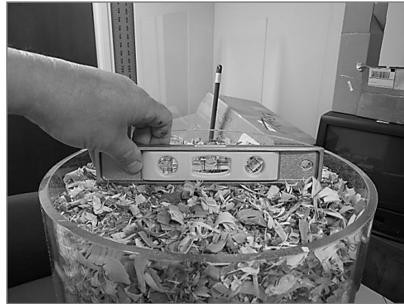
Exhibit 25. Checking Level. Checking the surface of large flake bedding for an approximation of a level condition.
