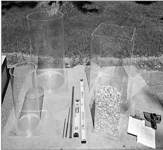
Exhibit 16. Test Measures Used in Study. The large test measures hold up to 279 L (10 cu ft) while the small measures hold up to 52 L (1.5 cu ft).
