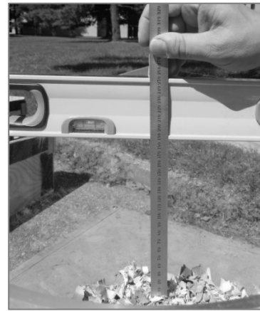
Figure 4. Showing how the ruler is placed on the bedding with the headspace method. The ruler is read from the bottom edge of a straight edge or level from a position that reduces parallax.
