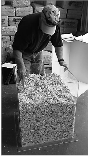
Exhibit 24. Leveling the Surface. Showing the use of a 150 mm mesh to level the surface of large flake bedding.
