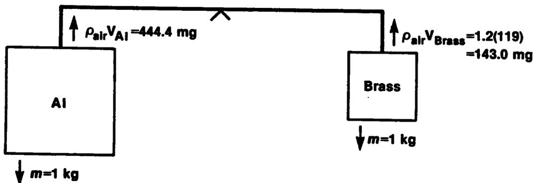
This means the aluminum weight appears to be 301.4 mg lighter than the brass weight. Hence the apparent mass of the aluminum weight versus brass is approximately
