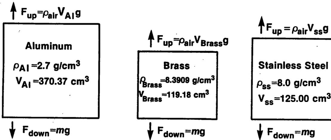
It can be seen that the larger the volume, the greater the upward force. Since gravity appears in all terms when the weights are intercompared, the gravity factor ( $g$ ) cancels.
