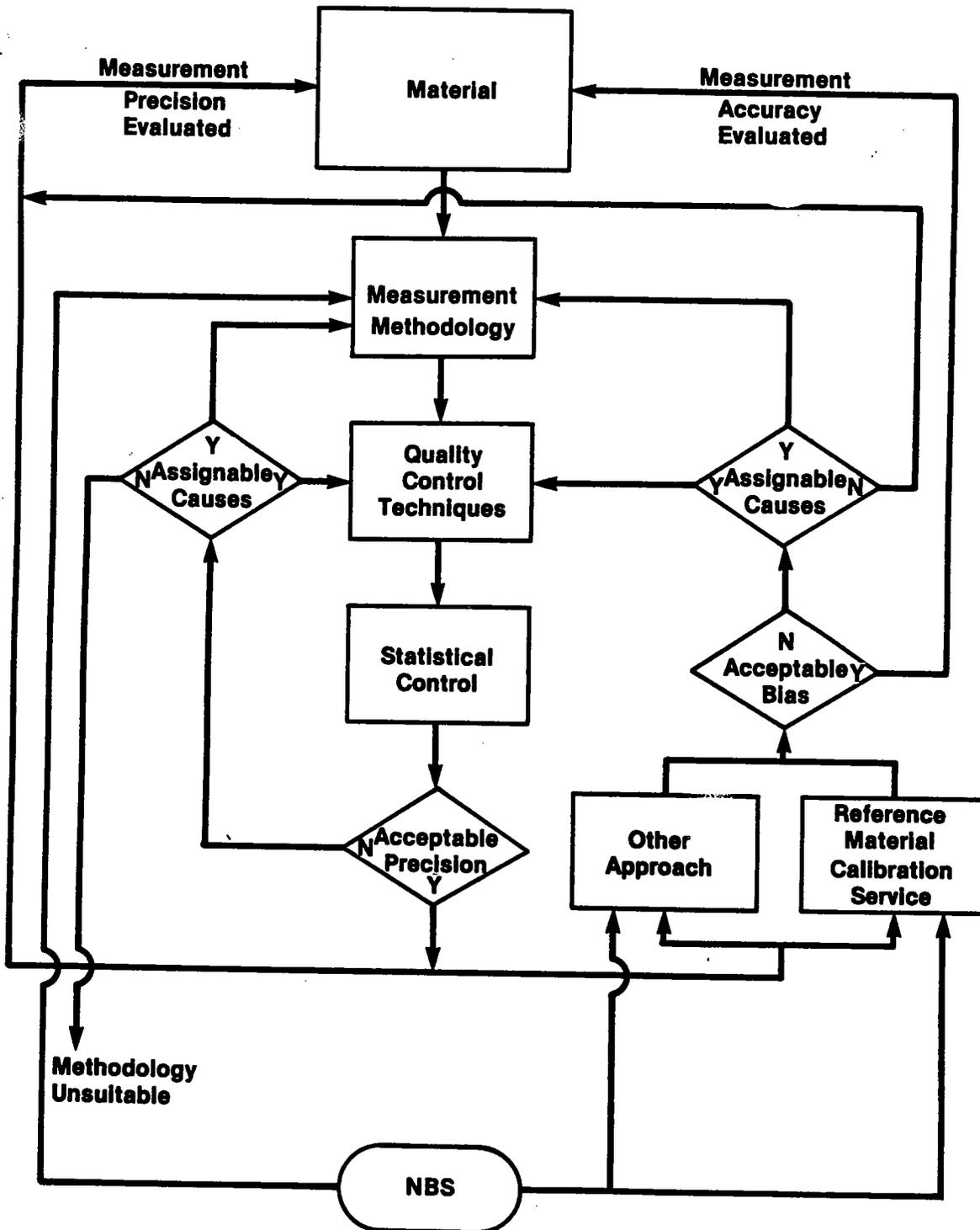
FIGURE 7.3 NBS SUPPORT FOR THE MEASUREMENT PROCESS
