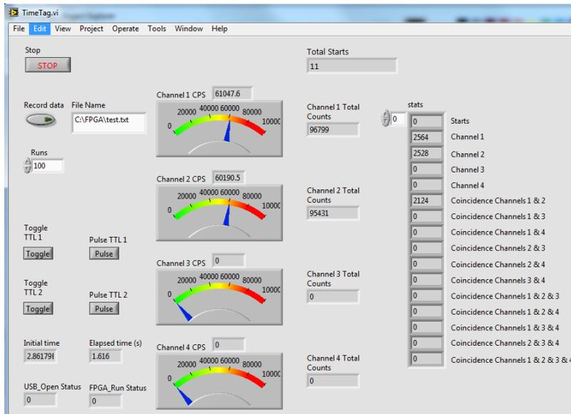
(b) TimeTag.vi registering a 50% duty cycle 60 kHz TTL signal.
