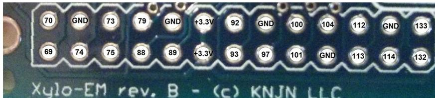
Figure 2: Xylo-EM Pinout. This information and a full board layout diagram can be found in the Xylo-EM documentation from knjn which comes with the board.
