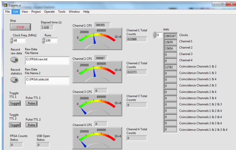
(a) Counts.vi registering a 50% duty cycle 400 kHz TTL signal.
