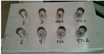
(a) Front panel BNC connector mounting.
