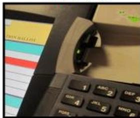
To start the voting process, insert the voter's card into the slot shown here.
