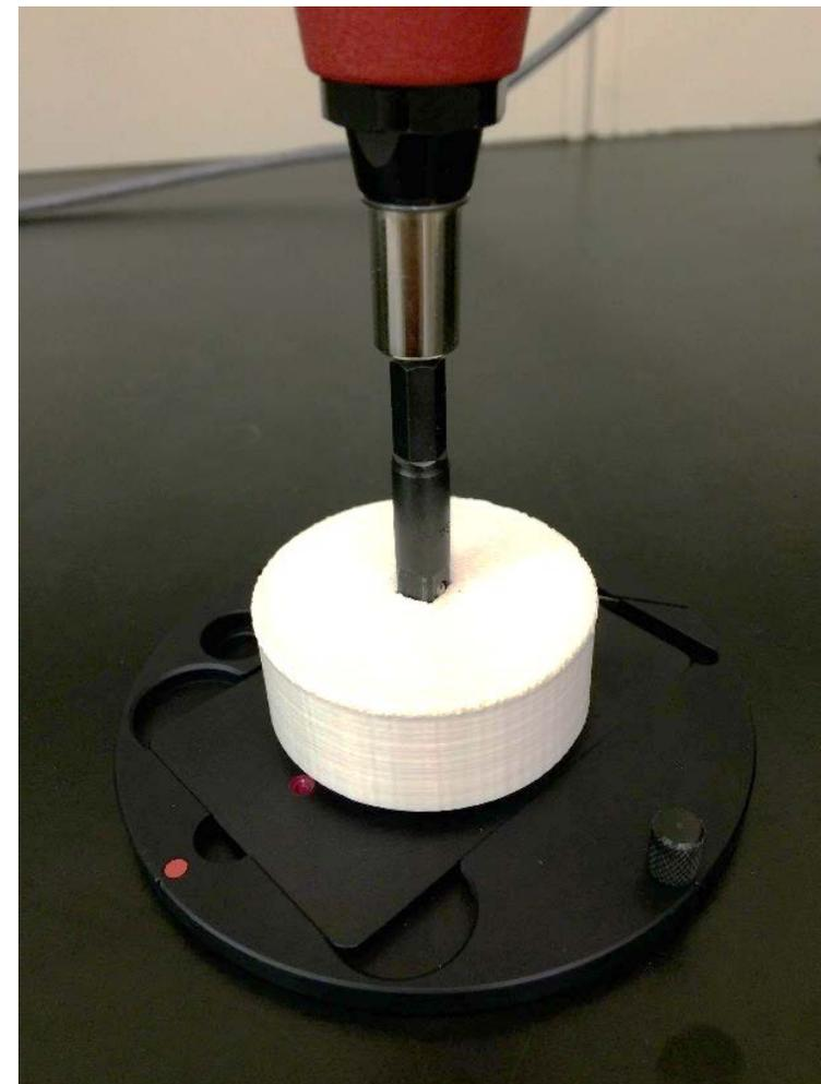
Adapter used with Torque Wrench
