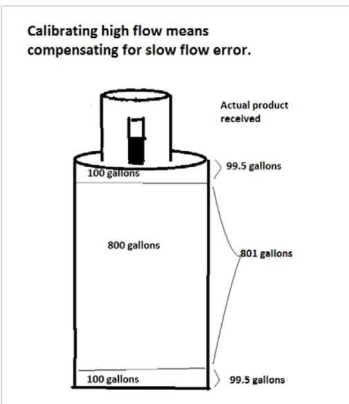
When calibrating at the normal and fallback speeds, the meter registers 200 gallons of product for the startup and shutdown, but actually delivers only 199 gallons. (99.5 gallons delivered for every 100 gallons registered at slow speed.) If the service technician calibrates the meter to zero at normal and fallback rates, the meter will actually deliver 801 gallons for every 800 gallons it registers at those rates.
