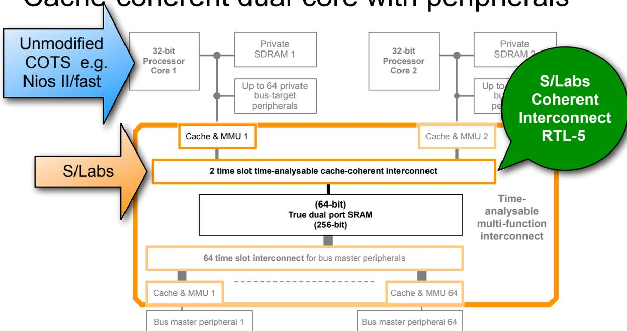
➔ The dual-core configuration adds S/Labs' time-analysable **cache-coherent** time slot based interconnect which has:
