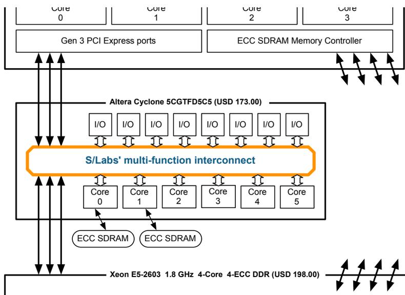
4. Implement our field-proven technology as a hard-macro in a SoC FPGA device or as dedicated ASIC chips
