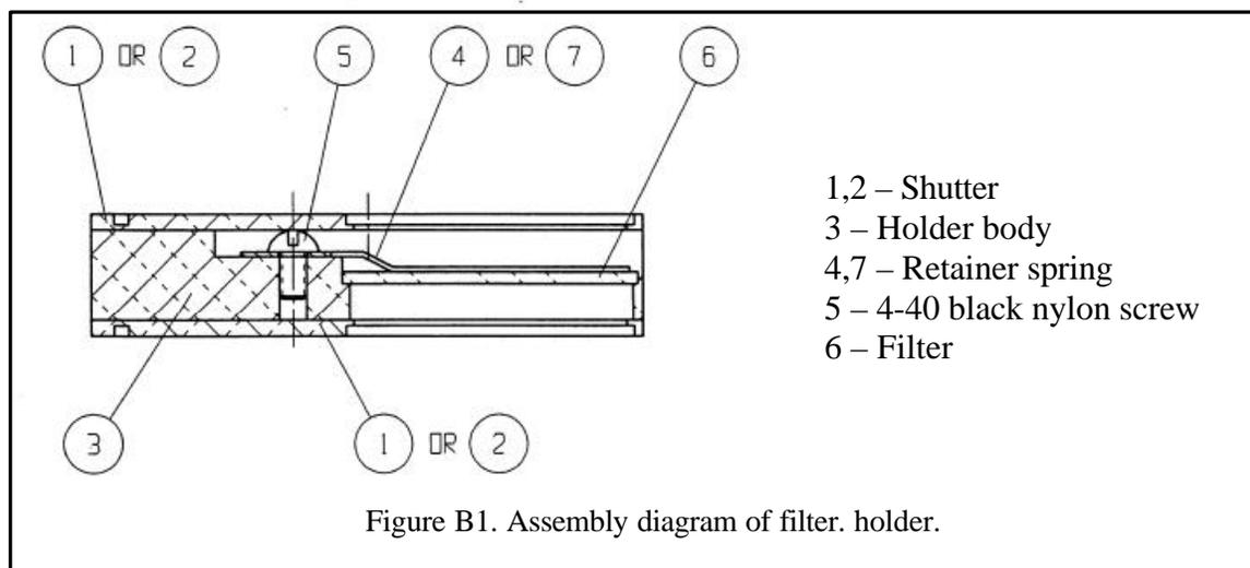
A noteworthy feature shown in Figure B2 (in the top views) is a tiny protrusion at the base of the holder, which keeps the filter from falling out of the holder. In the top right view of Figure B2, the dovetail grooves that hold the shutters in place may be seen. The shutters themselves are shown in Figure B3. They are made from black Delrin. Figure B4 shows the retaining clip, which is made from 0.5-mm thick aluminum.
