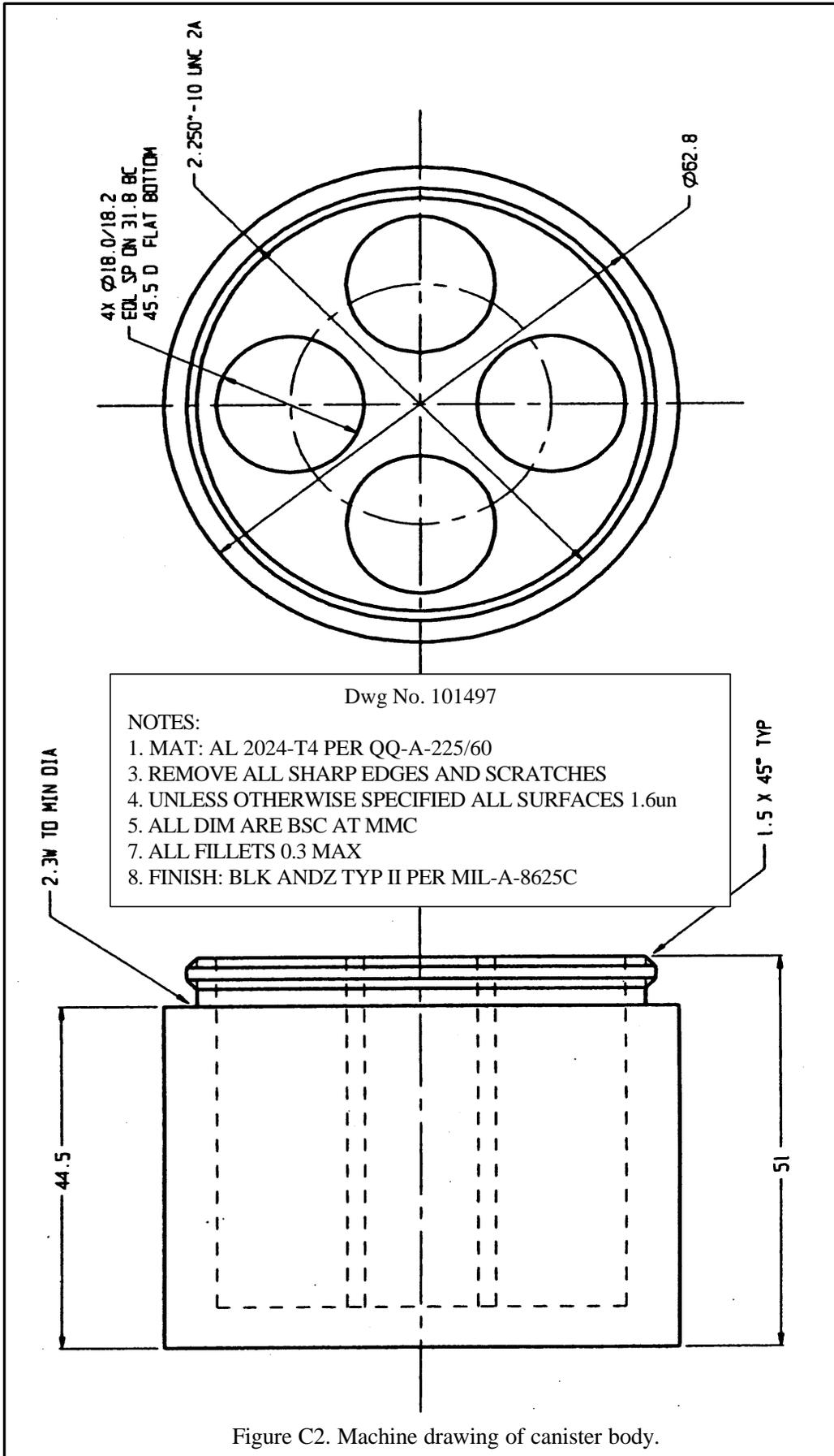
The default machining tolerances for the canister components are the same as for the filter holder components, and were given in Table B1.
