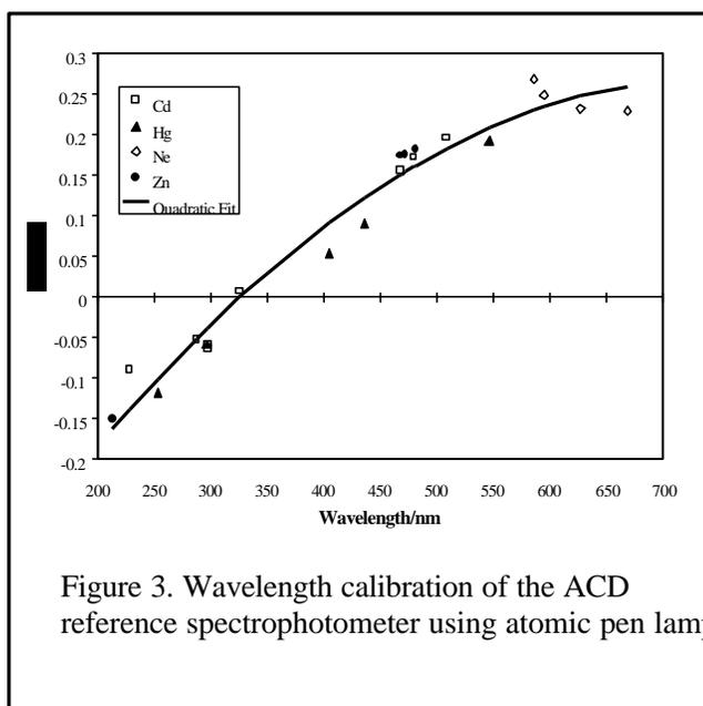
Figure 3. Wavelength calibration of the ACD reference spectrophotometer using atomic pen lamps.
