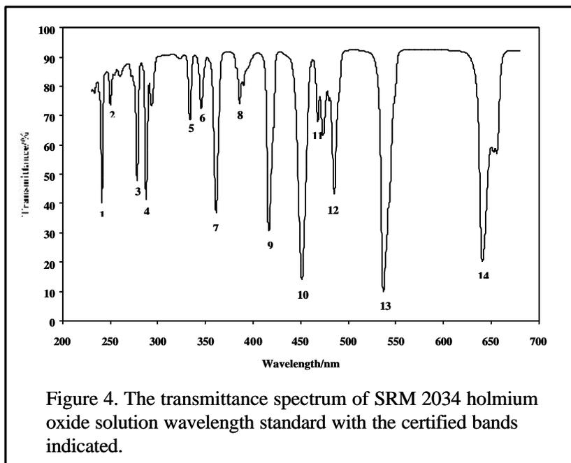
Figure 4. The transmittance spectrum of SRM 2034 holmium oxide solution wavelength standard with the certified bands indicated.
