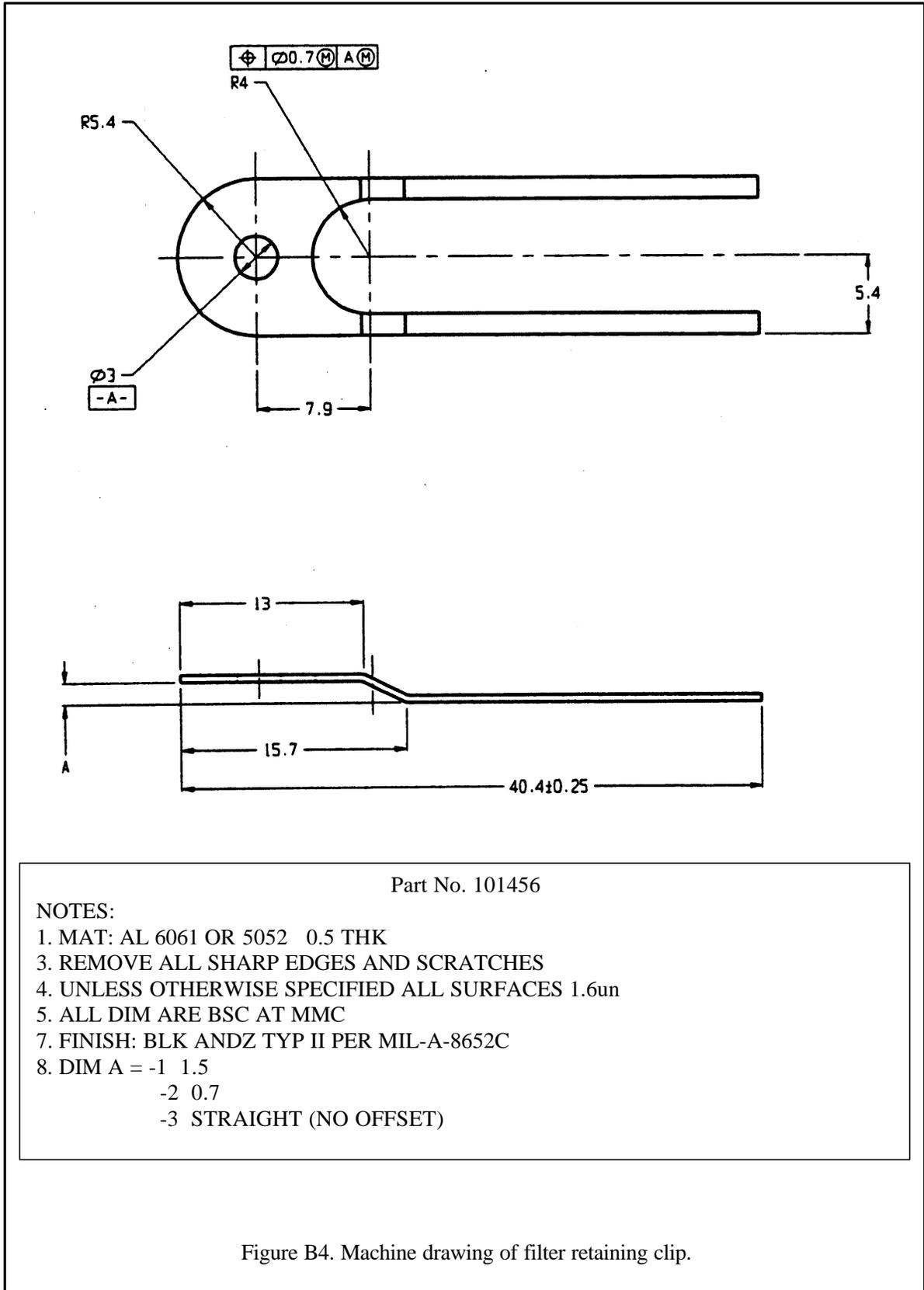
Figure B4. Machine drawing of filter retaining clip.
