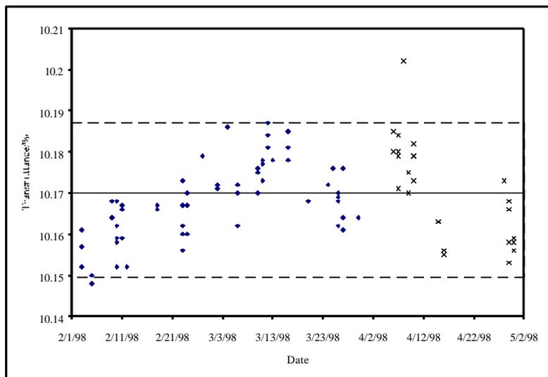
Figure 6. Control chart using SRM 930, filter 100-10 at 546.1 nm for the NIST ACD reference spectrophotometer.
