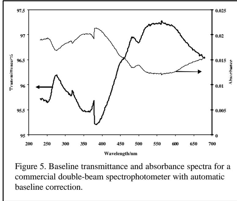
Figure 5. Baseline transmittance and absorbance spectra for a commercial double-beam spectrophotometer with automatic baseline correction.
