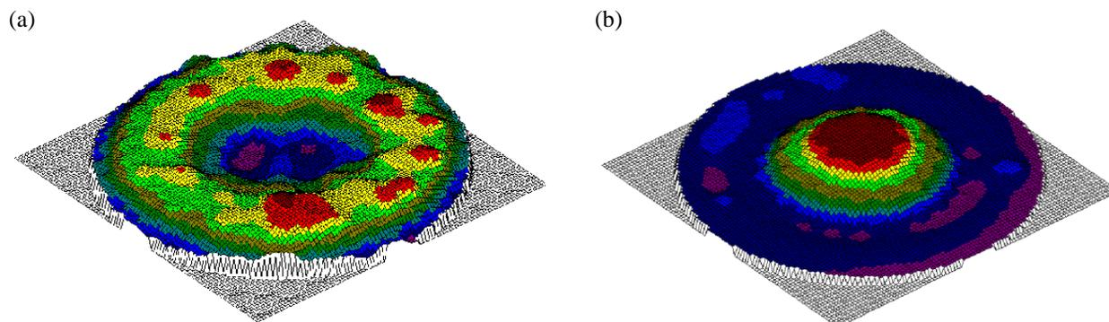
**FIGURE 1.** Rapid uniformity maps from a blanket SiGe epilayer on a 300 mm Si(001) wafer using (a) HRXRD for composition and (b) XRR for thickness. Thickness mapping is also possible with the HRXRD channel in the case of fully-strained epitaxial films.
