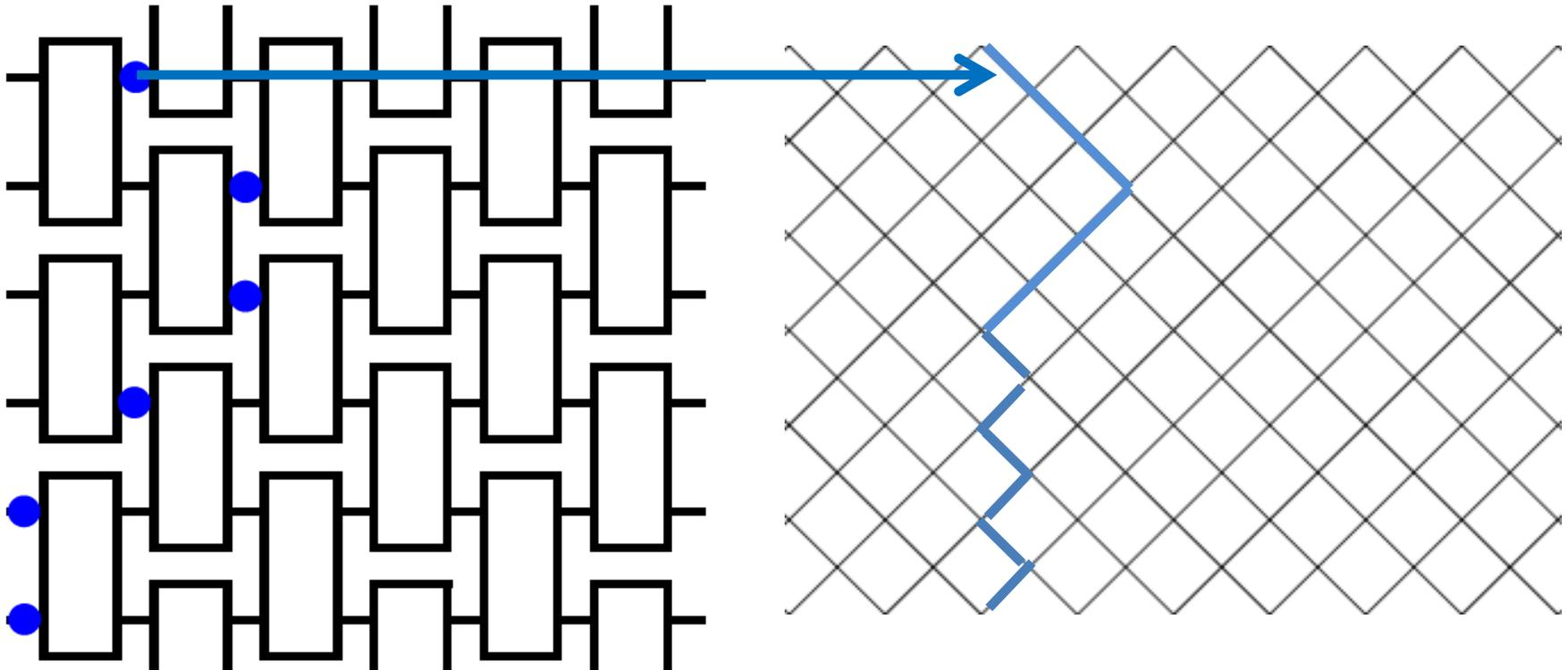
Picture on the right: each gate is represented as square and blue string is vertex in the graph. Points in time are on the edges. Strings (vertices) are connected by transitions  $\langle \leftrightarrow \rangle$ .
