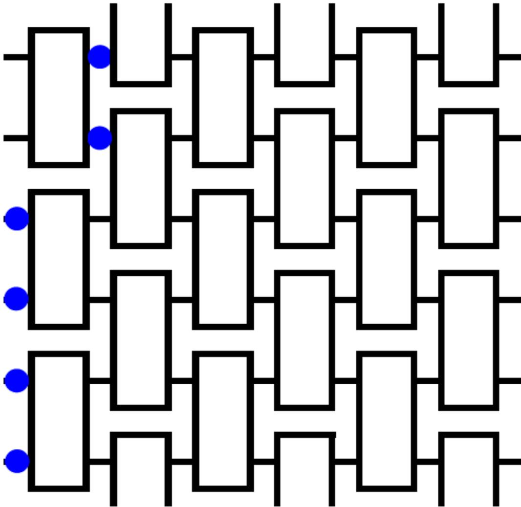
**Definition valid time-configuration  $t$**  (informally): for no pair of qubits interacting at time  $t$  in the circuit is the clock of one qubit past  $t$  and the clock of the other qubit before  $t$ .
