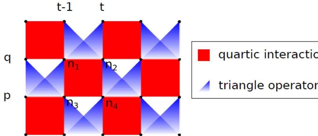
Figure 5: The black dots are fermionic sites, each with two modes (an  $\uparrow$  or  $\downarrow$  spin, say). The (red) squares represent the quartic gate interactions and the (blue) triangle operators penalize improper fermionic configurations (improper time-configuration). A (blue) triangle operator with top corner  $a$  and bottom corners  $b$  and  $c$  equals  $n_a(1 - n_b - n_c)$ . The lattice has periodic boundary conditions in both directions.
