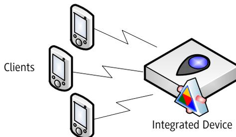
**Figure 3.** A physically integrated WS-Biometric Devices (WS-BD) implementation.
