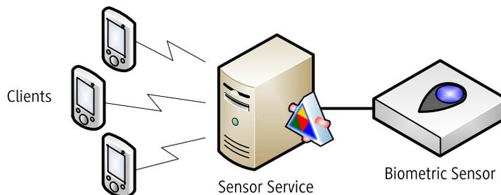
**Figure 2.** A physically separated WS-Biometric Devices (WS-BD) implementation.
