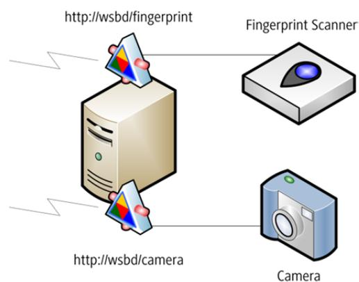
**Figure 4.** Independent sensors controlled by separate services
