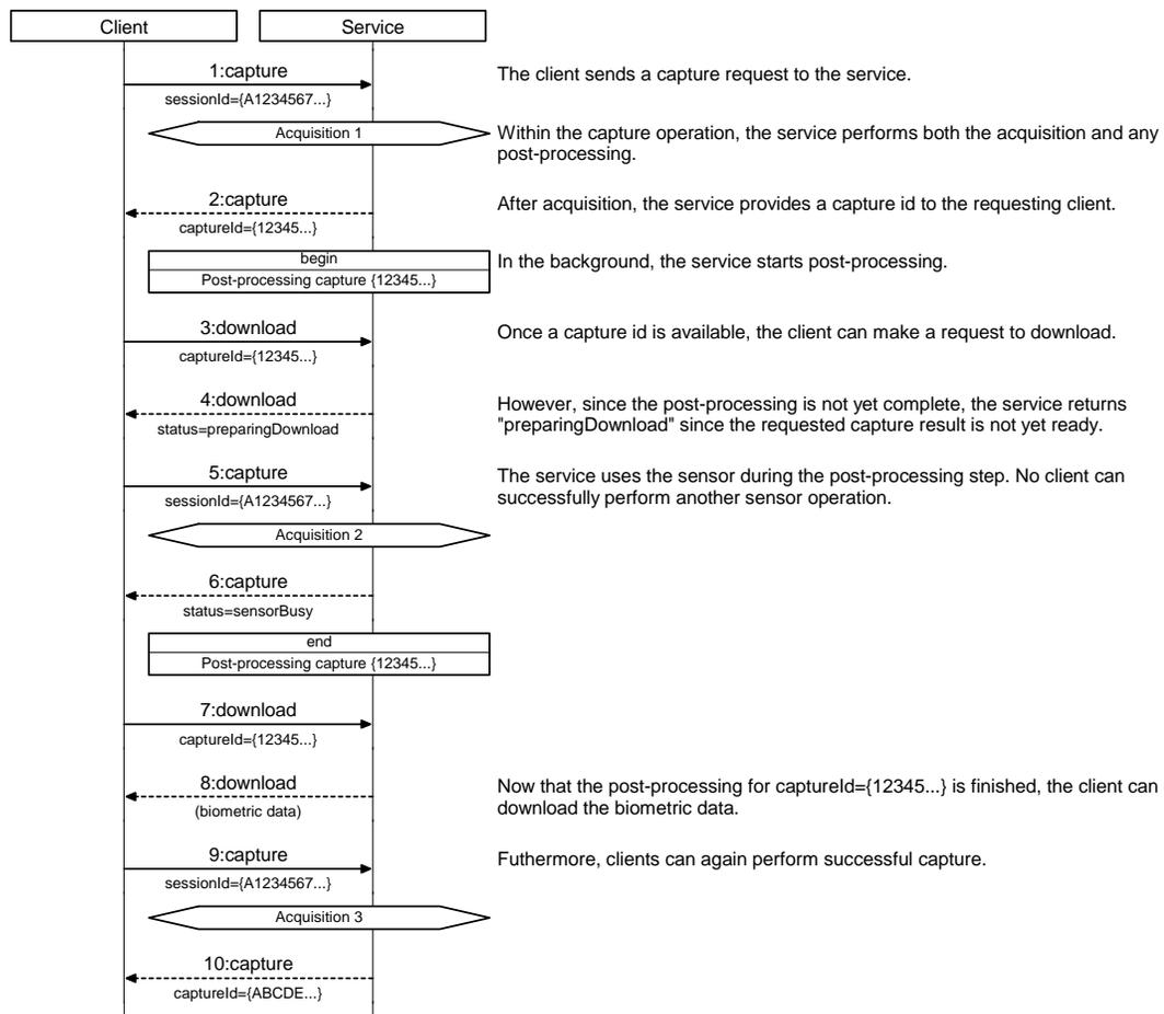
**Figure 11.** Example of capture with separate post-acquisition processing that does involve the target biometric sensor. Because the post-acquisition processing does not involve the target biometric sensor, it is available for sensor operations. Unless specified, the status of all returned operations is success.
