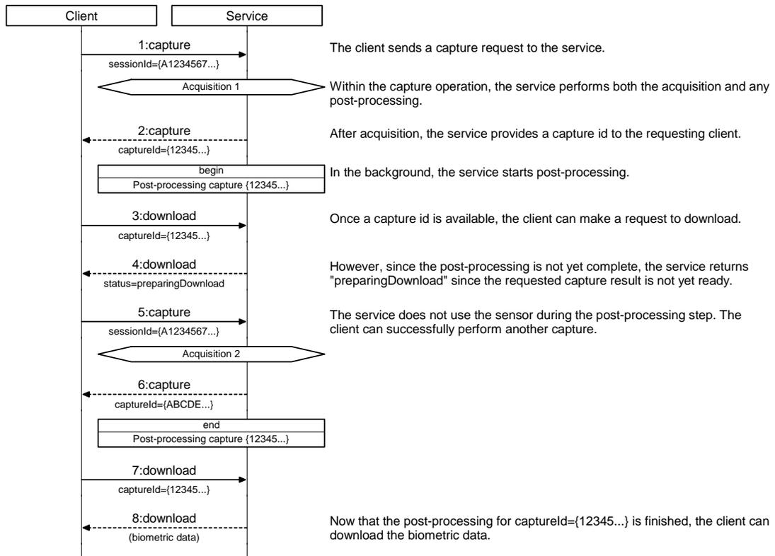
**Figure 10.** Example of capture with separate post-acquisition processing that does involve the target biometric sensor. Because the post-acquisition processing does not involve the target biometric sensor, it is available for sensor operations. Unless specified, the status of all returned operations is *success*.
