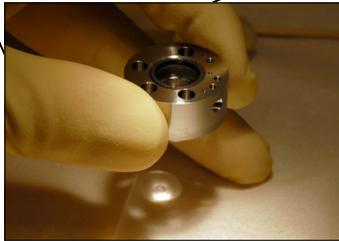
Prototype of the integrated Faraday cup and optical objective.
