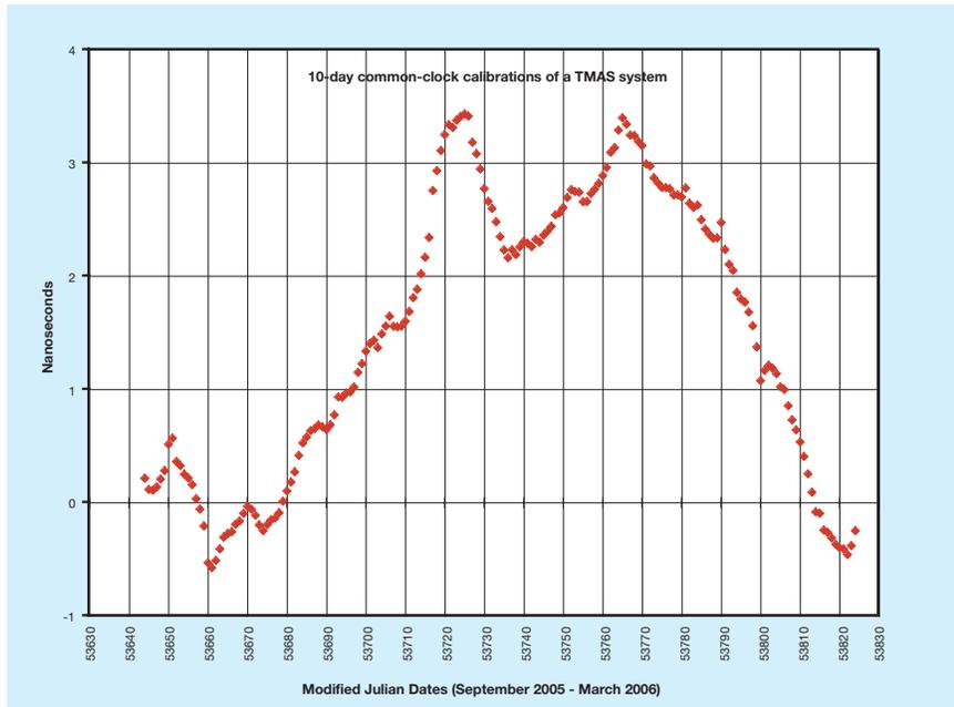
**Figure 9.** Results of consecutive 10-day common-clock calibrations made over a 190 day interval.
