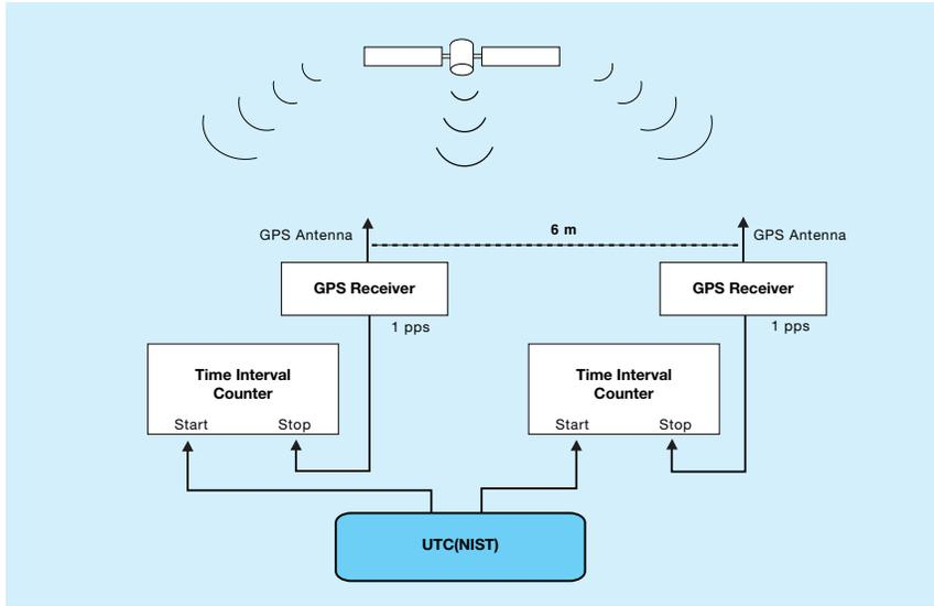
Figure 3. A common-view common-clock calibration of a TMAS measurement system.
