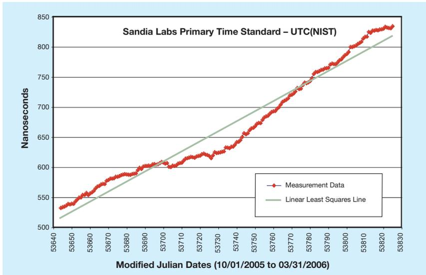
Figure 7. TMAS comparison (six months) between the time standard at Sandia and UTC(NIST).
