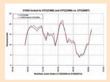
Figure 7. Comparison between UTC(CNM) time scale and CVDO locked to UTC(CNM).
