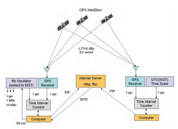
Figure 2. Schematic of the NISTDO system.
