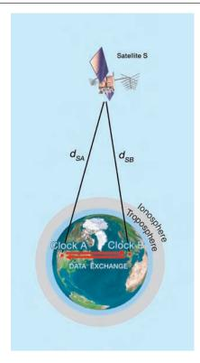
Figure 1. The common-view GPS measurement method.
