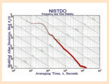
Figure 5. Frequency stability and time stability (diagonal lines) of NISTDO with respect to UTC(NIST).
