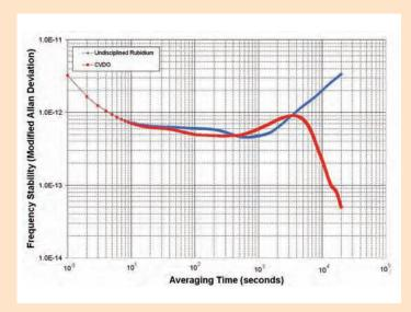
**Figure 6**. Frequency stability of NISTDO compared to undisciplined rubidium oscillator.
