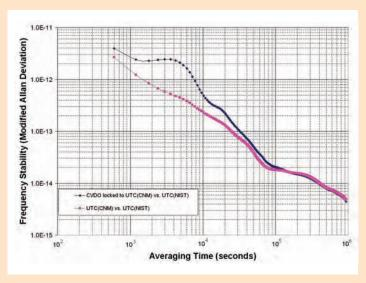
**Figure 8.** Stability comparison between UTC(CNM) time scale and rubidium locked to UTC(CNM).
