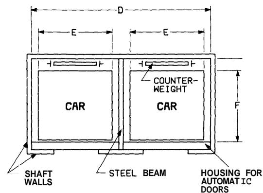
Fig. A1. Convention used for determination of  $A$ , and  $A_f$ .  $A = DG$  and  $A_f = DG - NEF$  where  $N = 1$  for a single car moving and  $N = 2$  for both cars moving together. Note that the area,  $A_f$ , does not include the small area between the car and the door housing because it is felt that the contribution of this area is insignificant.
