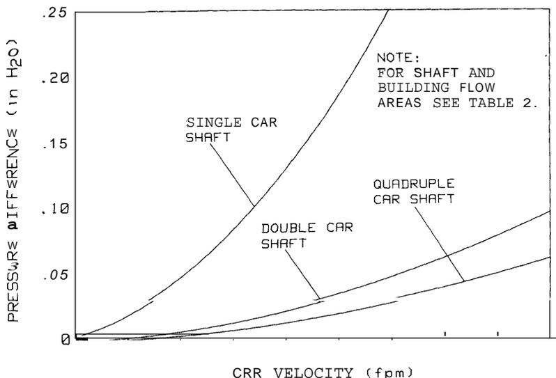
Fig. 3. Example pressure differences from building to elevator lobby due to piston effect. Conversion factors: 1 in H<sub>2</sub>O = 248.8 Pa; 1 fpm = 0.00508 ms<sup>-1</sup>.
