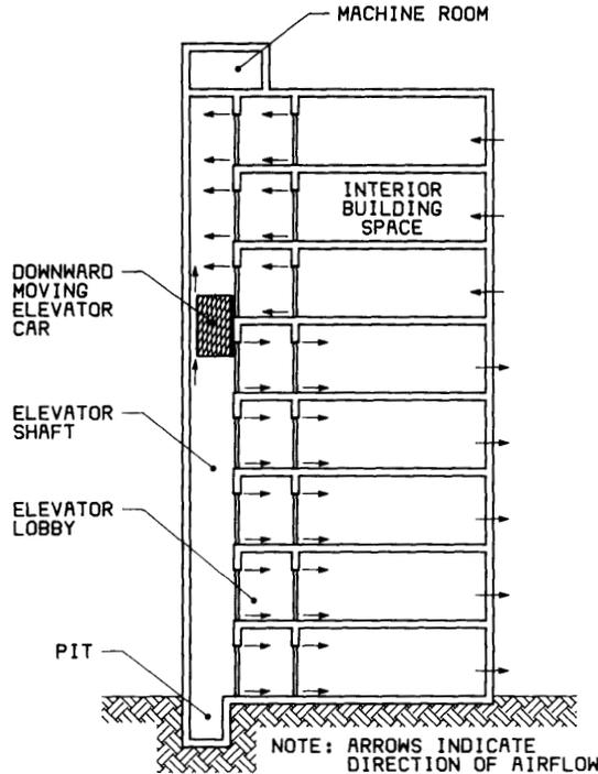
Fig. 1. Airflow due to downward movement of elevator car.
