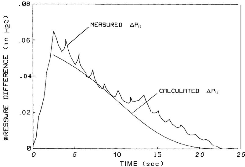
Fig. 2. Pressure difference,  $\Delta P_{ii}$ , across the elevator lobby of a Toronto hotel due to piston effect. Conversion factor: 1 in  $H_2O = 248.8$  Pa.
