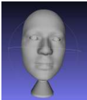
Figure 2 A 3D representation of an “average” human face with a mounting solution for model eyes which have specialized optical targets (Figure 3). The face model has a ¼-20 thread on the bottom to facilitate mounting to optical bench hardware to accurately control stand-off distance and presentation angle to evaluation devices
