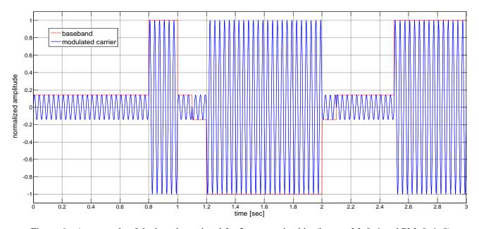
Figure 6 – An example of the broadcast signal for 3 consecutive bits (legacy: M, 0, 1 and PM: 0, 1, 0)
