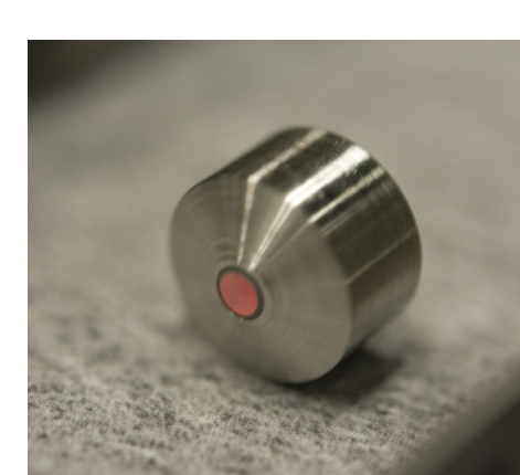
Ion is excited through the side of the cavity, at approximately 45^\circ to the vertical
