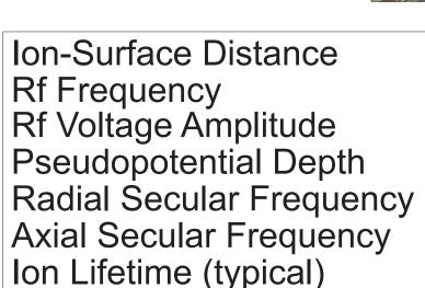
150 µm 25.8 MHz 112 to 223 V 47 to 188 meV 2.0 to 4.0 MHz 300 kHz to 1.2 MHz 5 min
