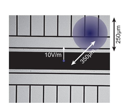
Trap appears to be fairly resistant to charging as ion sees no dielectric. 30 seconds of exposure with 10µW of 397nm light in the arrangement shown above produced a 10V/m field in the direction shown. Field returned to initial value after around 10 mins and was measured by looking at the induced micromotion. A more detailed study will follow.
