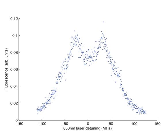
Scan of 850nm repumper that is 45deg out of the plane of trap in Trap 2.
