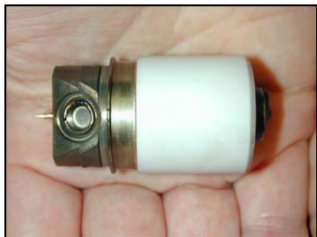
Integration in miniature X-ray tube (Oxford XTG Inc.)
