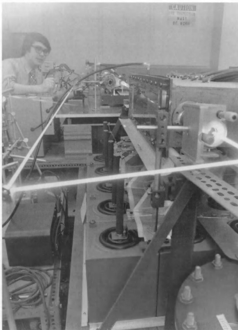
George H. Atkinson used a dye laser to detect free radicals, a technique that he developed at the National Bureau of Standards with Allan H. Laufer and Michael J. Kurylo.
