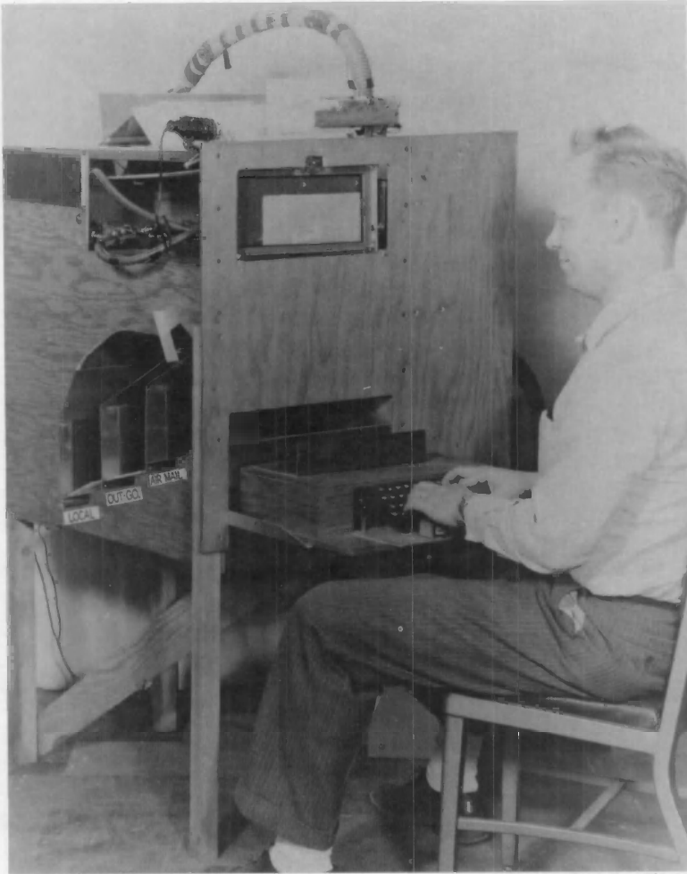
First model of a letter-coding station for an automatic mail sorting machine built by Rabinow Engineering Company under contract to NBS. Letters, one at a time, were presented to the operator who read the addresses, abbreviated their important parts, and typed the abbreviations onto the backs of the envelopes by means of a special printer. The printing code was in a binary form, and appeared in the form of "dot" or "no dot" on the envelope. The operator was John McDonald.
