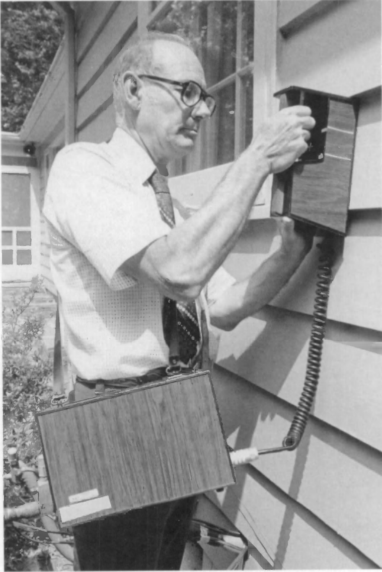
Philip A. Cramp, a chemist with the NBS Center for Building Technology, operated a portable X-ray-fluorescence instrument to measure lead levels on the exterior wall of a house.
