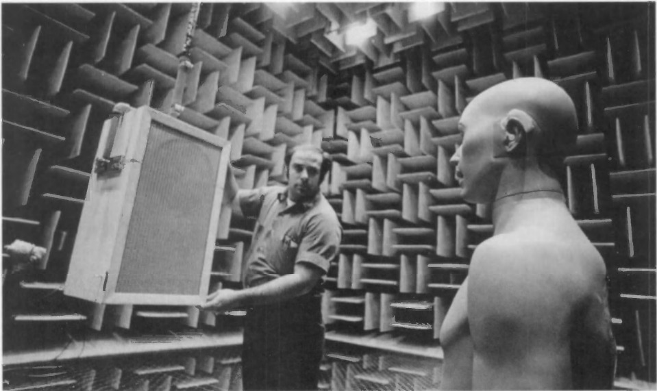
An anthropomorphic mannequin used for acoustic research at NBS "listened" through an over-the-ear hearing aid in an anechoic chamber as part of a testing program conducted for the Veterans Administration. Martin Bassin positioned the sound source.
