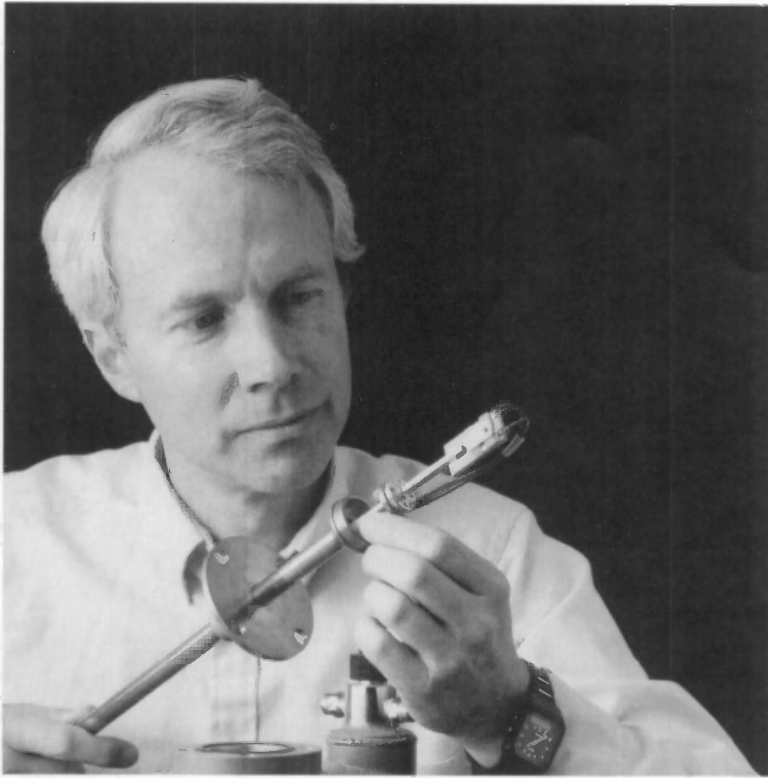
NIST electronics engineer Clark A. Hamilton examined the 1 V Josephson series array voltage standard. With about 3000 junctions, these NIST-fabricated integrated circuits are used in standards laboratories around the world.
