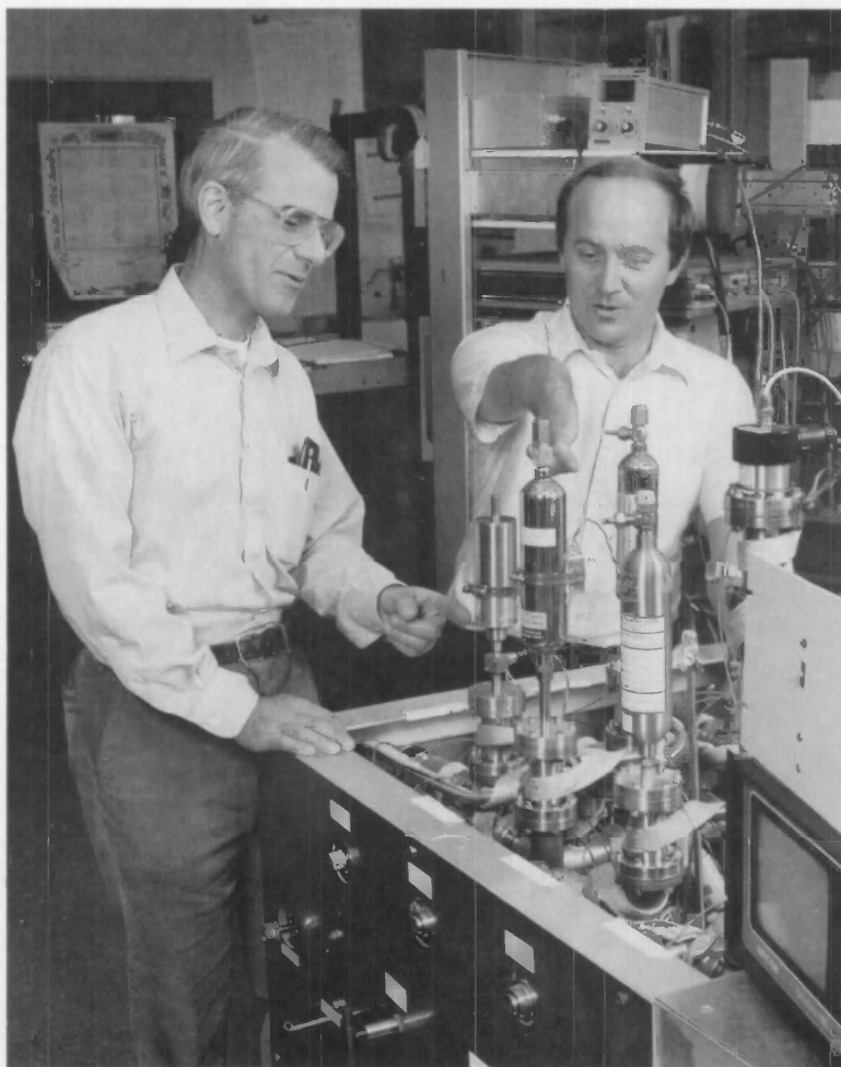
Richard Hyland (left) and Charles Ehrlich compared features of several calibrated leak artifacts mounted to the vacuum manifold of a new primary leak standard. Developed in the mid-1980s, the leak standard initially was used to provide calibrations for helium permeation leaks.
