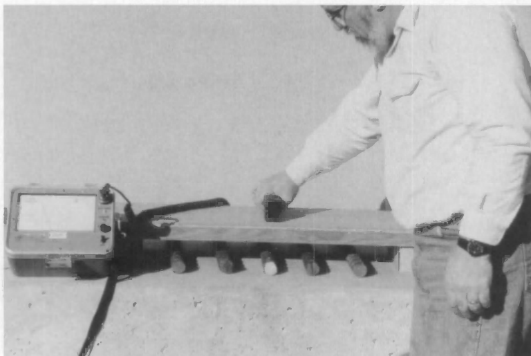
NIST Structures Division engineer Nicholas J. Carino operated a covermeter for locating reinforcing rods in reinforced concrete. The device operated by detecting magnetic reluctance.
