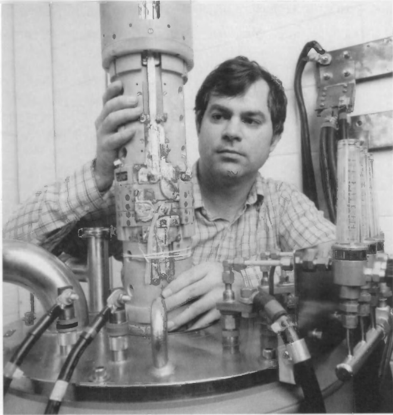
NIST physicist Loren F. Goodrich lowered a test cryostat containing a high-current niobium-titanium superconductor into a high-field magnet for critical current testing.
