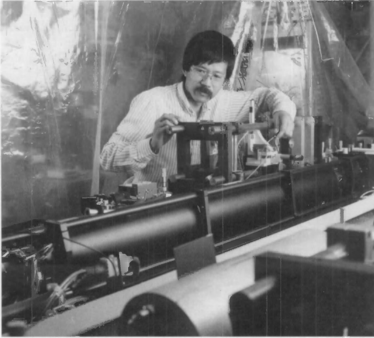
Wayne M. Itano adjusted an external frequency doubler, which was part of a laser setup for the mercury ion clock experiment.
