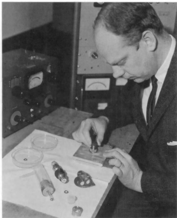
Martin G. Broadhurst cut leaf wafers for a 1968 study of the dielectric properties of foliage. The data were employed in the design of radio antennas for use in heavily wooded areas.
