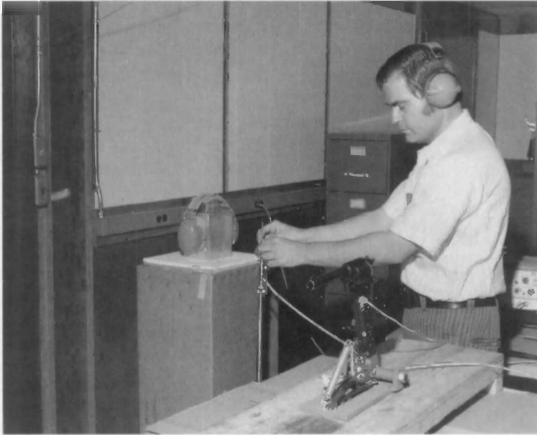
Physicist Michael T. Kobal of the NBS Sound Section developed a test to evaluate the effectiveness of hearing protectors used on firing ranges.
