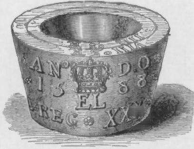
The standard troy pound of Queen Elizabeth, formed of 8-ounce and 4-ounce nesting weights.
