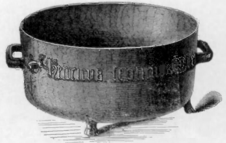
The Winchester bushel of Henry VII, a corn bushel, with a capacity of 2,150.5 cubic inches. This was the first English standard measure of capacity of which there is any cognizance.
