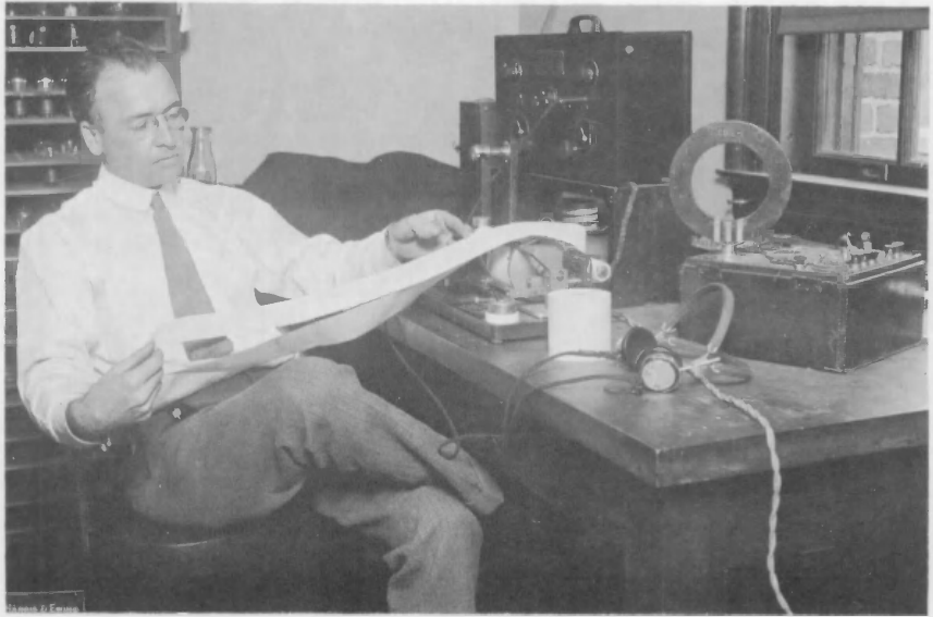
Dr. J. Howard Dellinger examines the continuous recording of super-power tests of station WGY, Schenectady. In 1926 when this picture was taken, WGY had been granted permission to broadcast regularly twice a week on 50,000 watts. WGY assisted the Bureau for a number of years in both its studies of radio interference and its compiling of radio propagation data.
