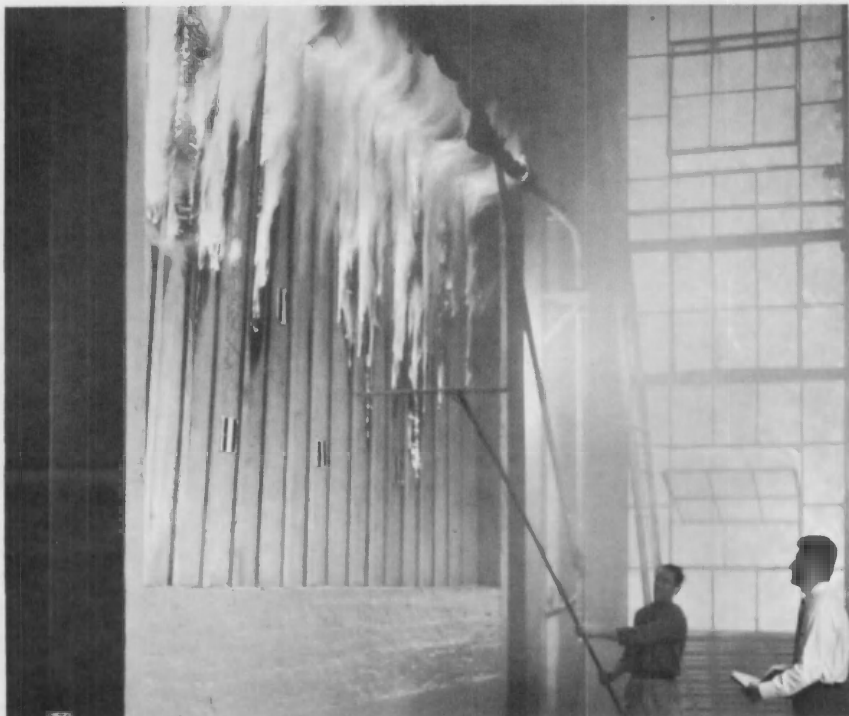
In this test of house wall fire resistance, the fire took 27 minutes to come through the Douglas fir siding as gas flames were applied to the other side. An instrument on the pole measures the bulge of the wall. (Picture by courtesy of the National Geographic Society.)
