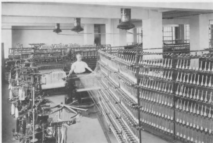
Above, the experimental rolling mill in the metallurgical division, a 16-inch mill equipped for rolling plates, rods, or bars, both hot and cold. Below, the NBS experimental cotton mill, acquired after the war, showing the knitting machine on the left and the creel (sets of bars with skewers for holding paying-off bobbins) on the right.
