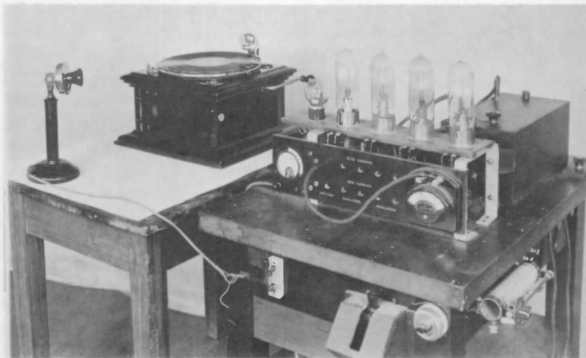
The phonograph playing into the high-power radiotelephone transmitter may be the experimental "broadcast station" pioneered by the Bureau. The date of the photograph is September 1920.
