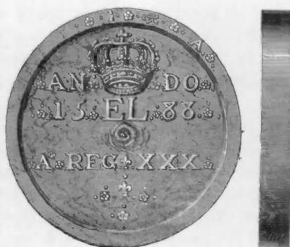
The standard avoirdupois pound of Queen Elizabeth I, which is believed to have originally weighed about 7,002 troy grains. It was used as a British standard from 1588 to 1825.
