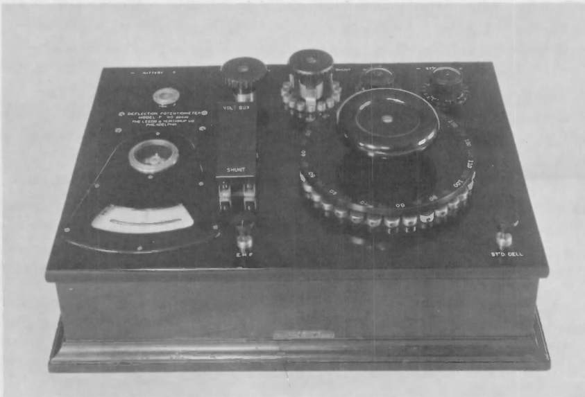
Dr. Brook's deflection potentiometer permitted the measurement of direct current and voltage more precisely than with any former laboratory indicating instrument. The potentiometer has come into wide use in the manufacture and rapid checking of precise indicating instruments with direct reference to a standard cell.
