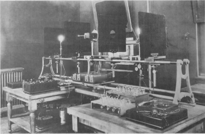
Laboratory setup for testing the candlepower of incandescent lamps about 1910. This was the brightness test, using a horizontal bar photometer.
