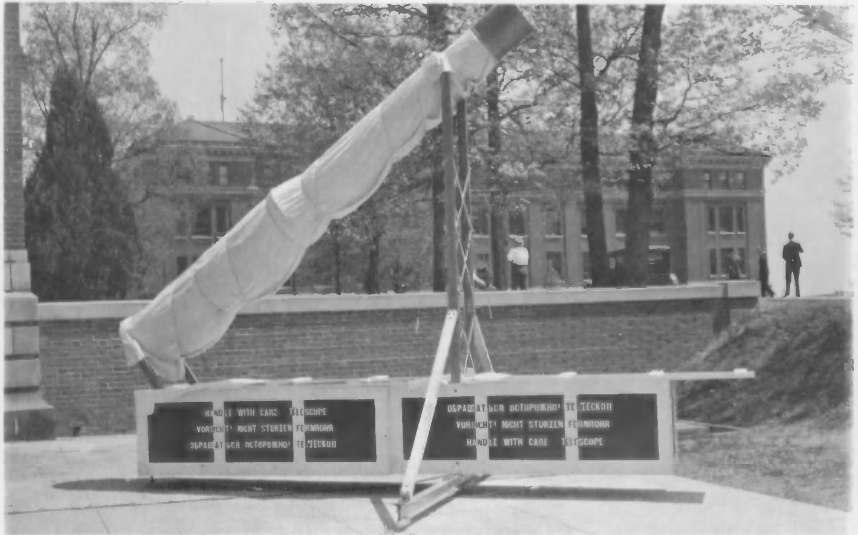
Dr. Gardner's specially designed camera for photographing the solar corona. It was used at Ak Bulak in Asiatic Russia in 1936 and at Canton Island in the South Pacific in 1937. The lens was made at NBS from optical glass poured in the Bureau glass plant.
