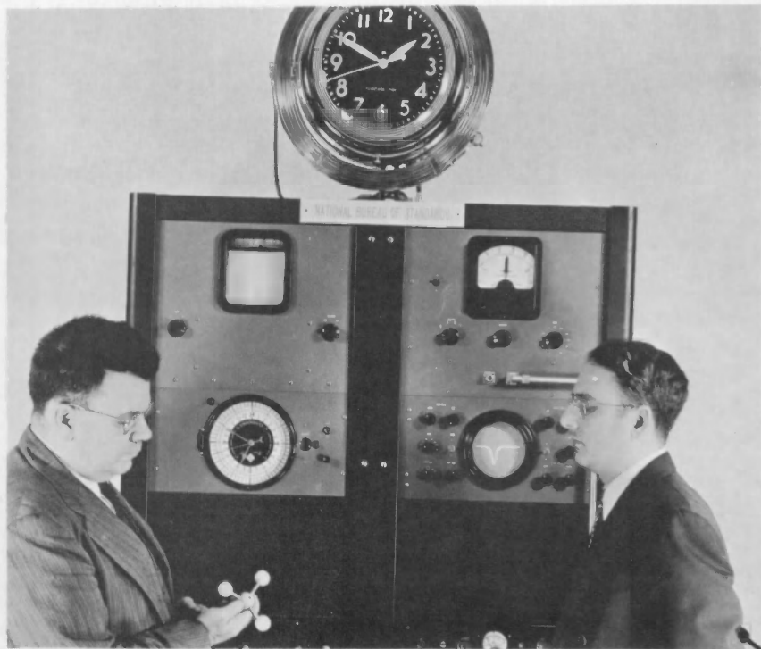
Dr. Condon and Dr. Harold Lyons with the first atomic beam clock. It operated with an ammonia-regulated quartz crystal and ran with a constancy of one part in 20 million.
