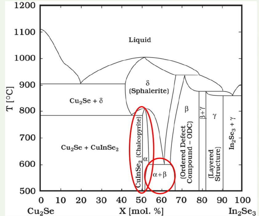
T-X section of the phase diagram along the Cu<sub>2</sub>Se-In<sub>2</sub>Se<sub>3</sub> pseudobinary section of the Cu-In-Se chemical system.
