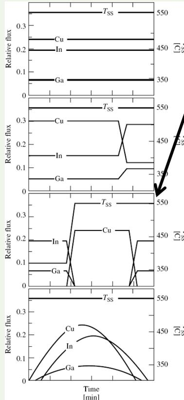
Relative metal fluxes and substrate temperature for different coevaporation processes; a constant Se flux is supplied.
