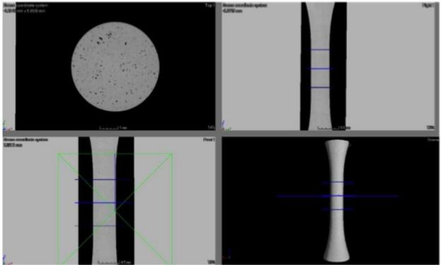
Figure 1: Example of CT scan of the defects in a fatigue specimen
