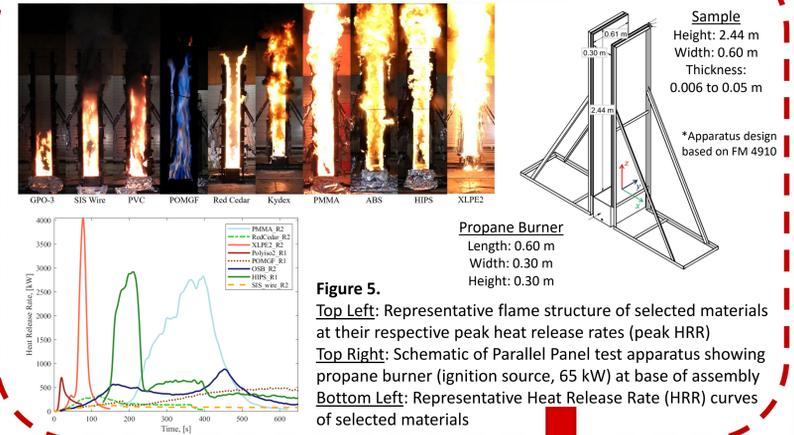
Figure 5. Top Left: Representative flame structure of selected materials at their respective peak heat release rates (peak HRR). Top Right: Schematic of Parallel Panel test apparatus showing propane burner (ignition source, 65 kW) at base of assembly. Bottom Left: Representative Heat Release Rate (HRR) curves of selected materials
