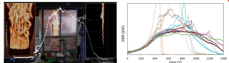
Figure 4. Top Left: Peak fire size during burning of 0.5 m tall, 0.2 m wide samples; enclosure dimensions 1.2 m wide, 1.8 m tall. Bottom Left: Well-characterized ignition source; repeatable between upward (+90°), downward (-90°), and horizontal (0°) flame spread. Top Right: Impact of sample variability, deformation, and melt pool formation (and pool burning) on measured fire development
