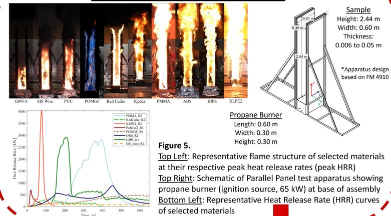
Figure 5. **Top Left:** Representative flame structure of selected materials at their respective peak heat release rates (peak HRR)
