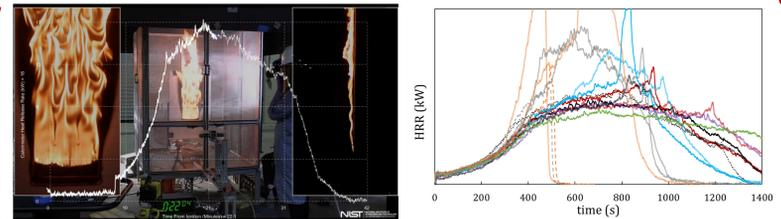
Figure 4. **Top Left:** Peak fire size during burning of 0.5 m tall, 0.2 m wide samples; enclosure dimensions 1.2 m wide, 1.8 m tall
