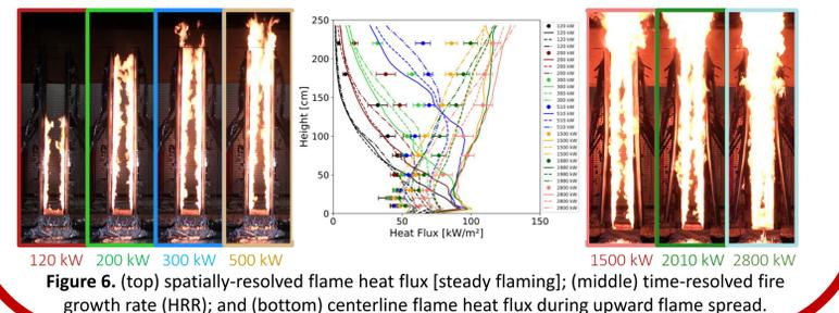
Figure 6. (top) spatially-resolved flame heat flux [steady flaming]; (middle) time-resolved fire growth rate (HRR); and (bottom) centerline flame heat flux during upward flame spread.
