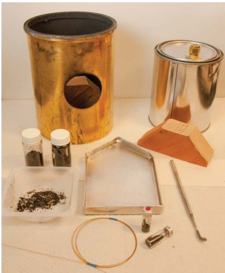
Shown here are the tools for testing arson samples using NIST's new PLOT capillary method. Clockwise from top are a test chimney with burned sample of Douglas Fir (used in test burns), paint can equipped with a septum cap, test sample of Douglas Fir, scraper, collection tray, fire debris samples, then at the bottom a PLOT capillary and two containers used with the capillary.
