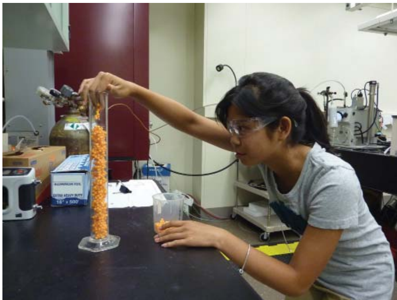
High school student Jessica Young checking the packing density of random aggregates of plastic spheres in a cylinder. Young's work as a summer intern at NIST contributed to a paper arguing that rigid aggregates like those she's testing tend to clump together at roughly the same density regardless of scale, from microscopic soot to large comets.
