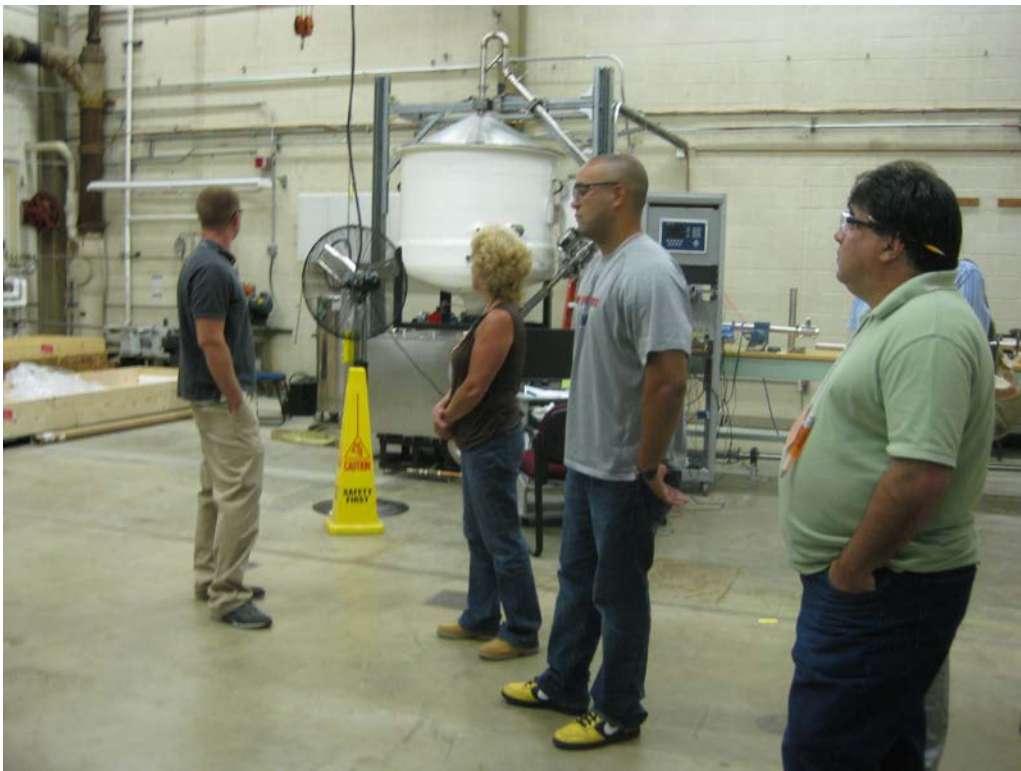
The white tanks are filled with purified water and are used to calibrate liquid flow meters used in the petrochemical industry, for aircraft engine manufacturers, the biotech industry, the semiconductor industry, and others.
