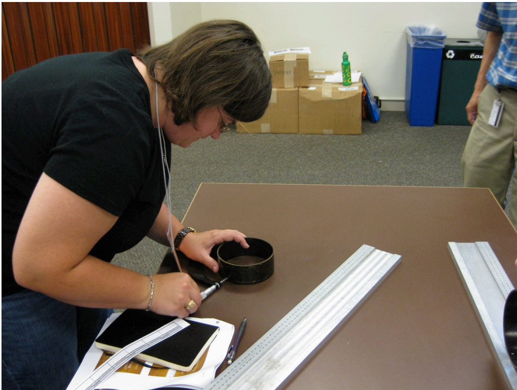
After Hung-kung's lesson, Loryn has no trouble using the calipers to accurately measure the diameter of the copper ring.
