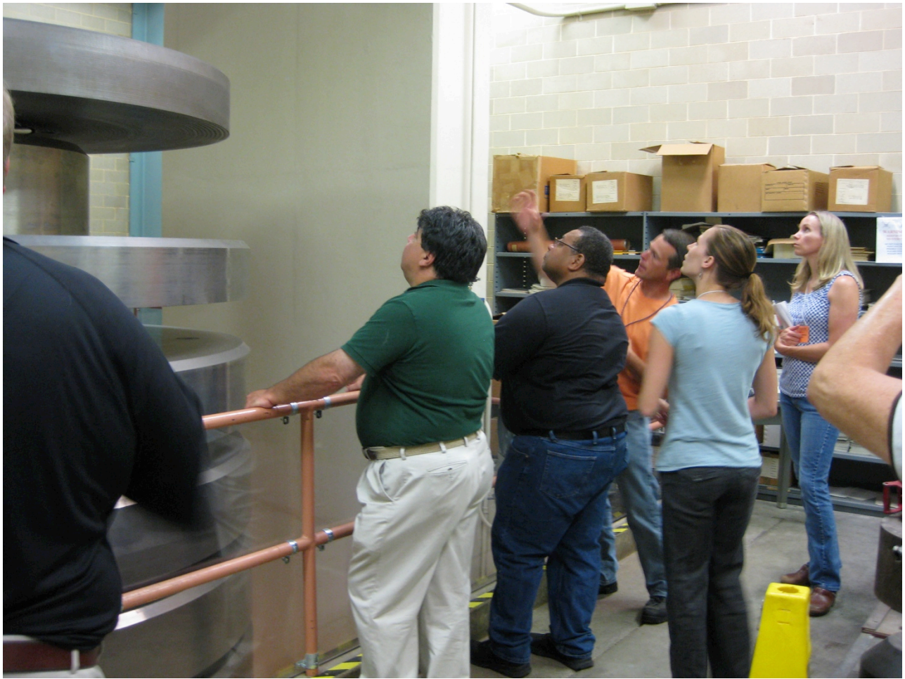
On the next level down of the 1,000,000 lbf (4.4 MN) Deadweight Test Machine are the million pounds worth of weights, an impressive sight. This is the only machine in the world with a million pounds worth of dead weight.
