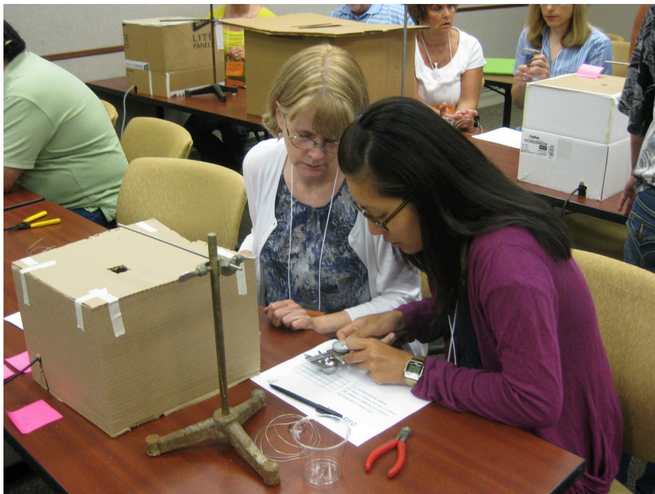
Martha and Jessica work to measure the diameter of the steel ball with calipers. (The cardboard box is a shield over the balance, designed to protect the balance from drafts, a source of uncertainty.)
