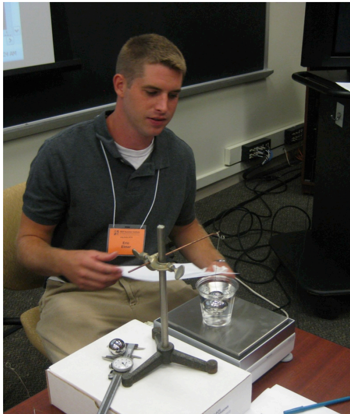
Eric measures the apparent mass of the steel ball suspended in water.
