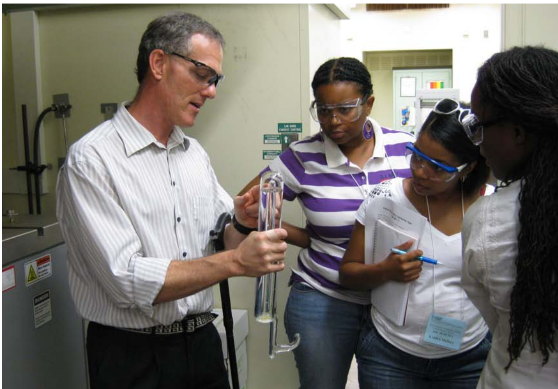
Greg demonstrates a water hammer for measuring the triple point of water. The device has very little air in it and so when the water moves from one end to the other the water “hammers” the other end with an audible thunk.
