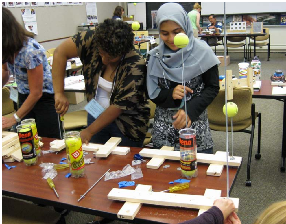
Another group works to build the reverse pendulums, designed to show how the natural frequency of earthquake waves resonates with buildings of a certain height.
