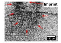
The image quality map of the cross section (above) shows that the deformation is detected via EBSD pattern quality mapping to a depth of about 520 µm beneath the bottom of the imprint. A criminal would therefore have to remove about 760 µm of material (140 µm imprint, 520 µm subsurface damage) to render a serial number undetectable by EBSD.
