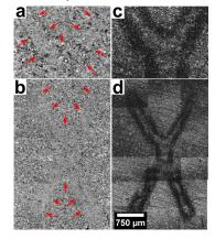
The imprint is faintly visible in the forward scattered image and very clearly visible in the EBSD pattern quality map. Low pattern quality in areas with sub-surface damage reveal the image of the stamped letter X.
