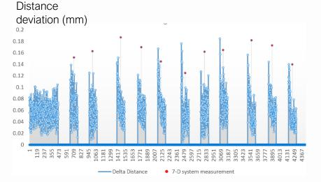
TCP deviations: 7-D system measured vs. calculated deviations from controller actual joint positions minus target joint positions
