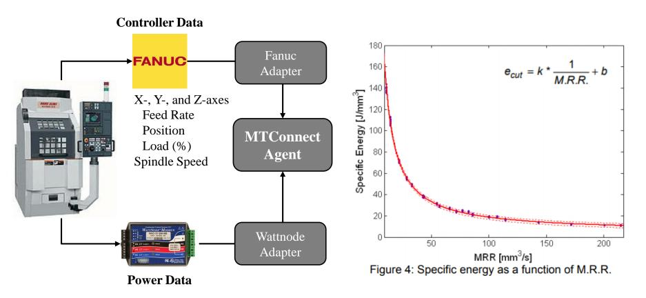
Diaz et al. (2011) "Energy consumption characterization and reduction strategies for milling machine tool use"
