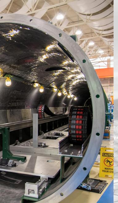
Credit: Fran Webber - Custom designed and built at NIST, the very small angle neutron scattering (vSANS) instrument at the Center for Neutron Research
