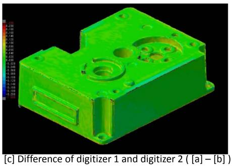
Difference between [a] and [b] is less than 0.05mm
