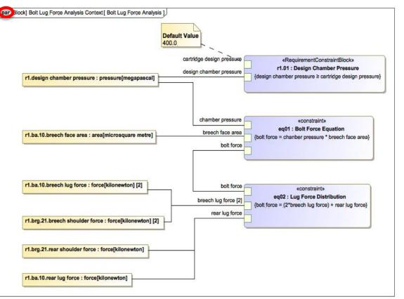
SysML parametric models are *acausal*:
