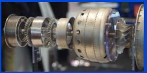
First 3D printed jet engine demo. Courtesy GE.
