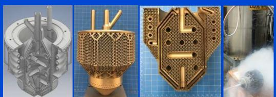
Cryo Heat Exchanger-Injector-Condenser Demo
