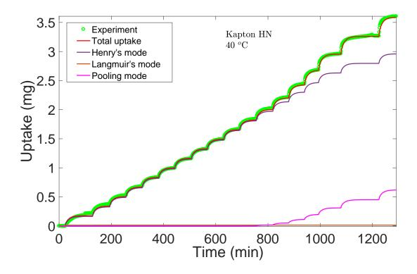
Fig 1: Experiments and modeling results of dynamic moisture uptake by Kapton HN at a range of relative humidities at 40°C.
