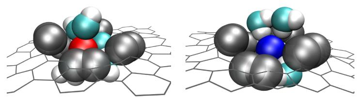
A potassium ion (red sphere, left image) and a chloride ion (blue sphere, right image) crossing a graphene pore both manage to retain many of their associated water molecules—represented by the bound oxygen (cyan) and hydrogen (white) spheres—despite the small size of the pore. Credit: NIST
