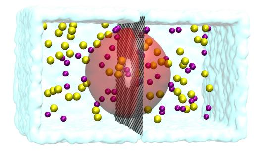
Schematic of a graphene nanopore shows an ionic solution partitioned by a graphene monolayer (gray, honeycomb membrane). The purple spheres are potassium ions and the yellow spheres are chloride ions with red indicating the access region. Credit: NIST
