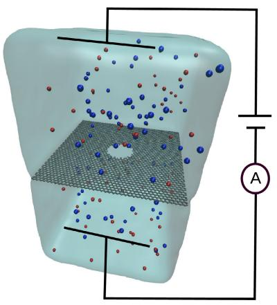
A voltage applied across a graphene nanopore drives an ionic current. When the pore is sufficiently small the ions must shed some of the attached water molecule in order to fit through the pore. Credit: NIST
