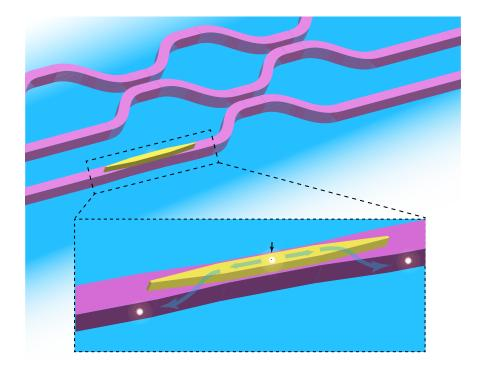
The architecture of this hybrid quantum photonic circuit is among the first to combine on a single chip a reliable generator of individual photons—a quantum dot (red dot), here embedded in gallium arsenide (yellow)—with passive elements such as a low-loss waveguide (purple) that transports the photons Credit: NIST
