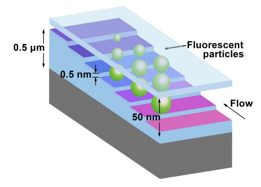
A nanofluidic staircase machined with subnanometer precision by a focused ion beam separates nanoparticles by size. The device is also a reference material to accurately measure nanoparticle size and compare it to optical brightness, which could aid in the quality control of consumer products. Credit: NIST
