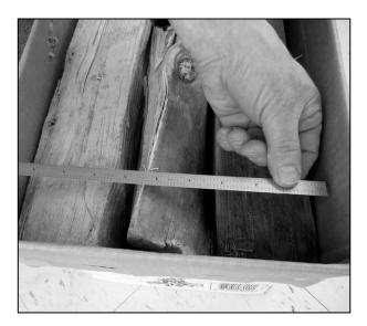
Figure 3-10a. Measuring the Width of the Firewood in a Box.
