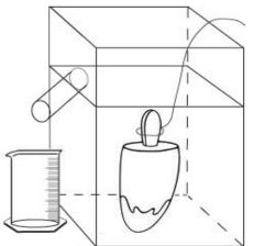
**Note:** This displacement vessel can be constructed or similar devices may be obtained from any laboratory equipment or science education supplier. The U.S. Department of Commerce does not endorse or recommend any particular device over similar commercially available products from other manufacturers.
