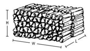
Figure 3-11. A Cord of Wood. A cord of wood measures 4 ft (height)  $\times$  4 ft (width)  $\times$  8 ft (length).
