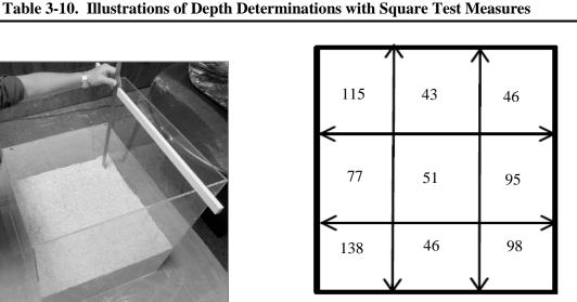
**Illustration 2. Measurement Grid for Headspace Measurement Procedure.**
