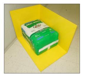
Figure 3-1. Dimensional Measuring Frame.
