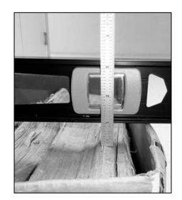
Figure 3-9a. Examples of the Headspace Measurement.
