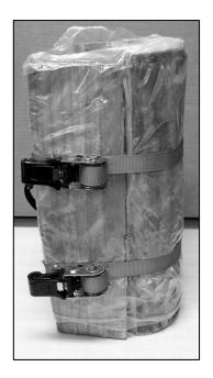
Figure 3-14. Bundle with Straps Placed at 10 cm (4 in).
