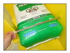
Figure 3-4. Length Measurement.
