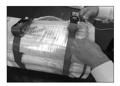
Figure 3-17. Strapping the Ends of a Bundle.
