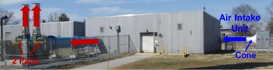
A Facility Designed to Assess the Flow Measurement Accuracy of CEMS and RATA
