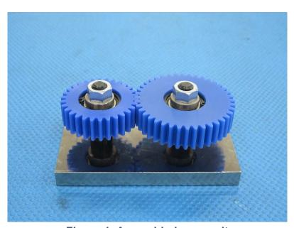
Figure 1. Assembled gear unit
